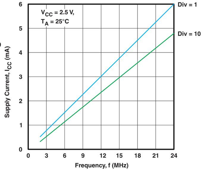
Figure 10. Supply Current vs Frequency (V<sub>CC</sub> = 2.5 V)
