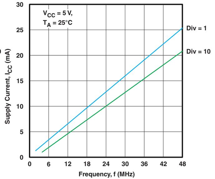
Figure 12. Supply Current vs Frequency (V<sub>CC</sub> = 5 V)
