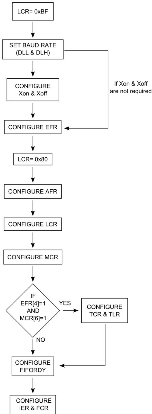
Figure 35. Diagram of the Generic Configuration Process
