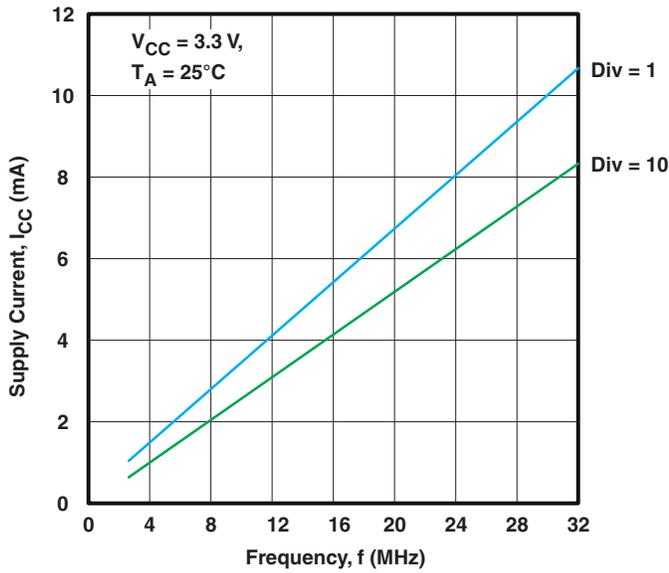
Figure 11. Supply Current vs Frequency (V<sub>CC</sub> = 3.3 V)
