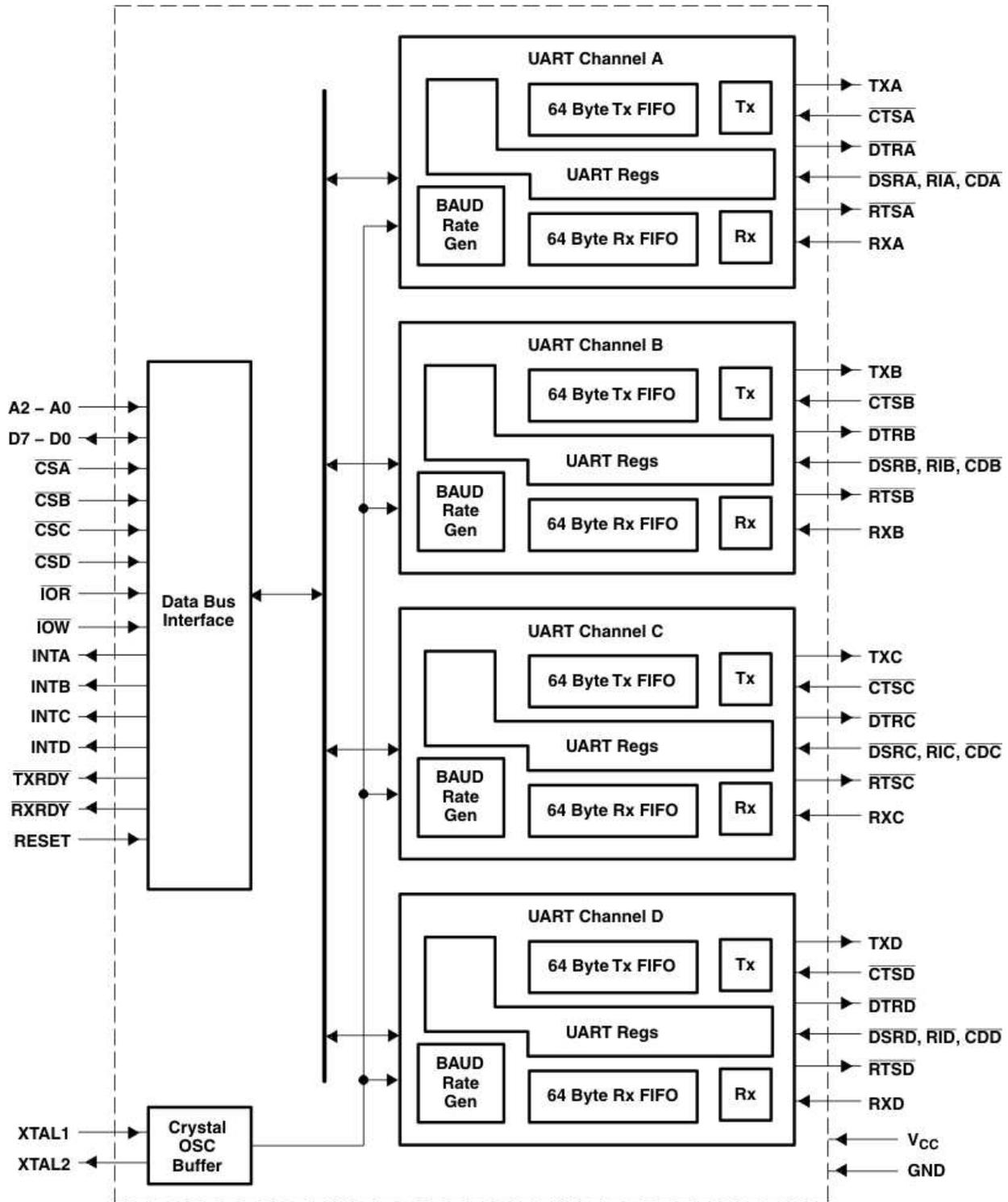
NOTE:  $\overline{\text{RXRDY}}$  and  $\overline{\text{TXRDY}}$  functionality is not supported in the TL16C754CPM device.
