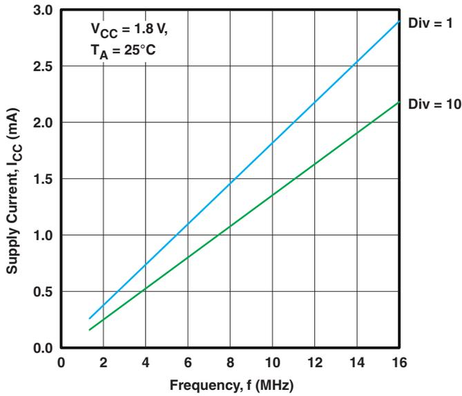
Figure 9. Supply Current vs Frequency (V<sub>CC</sub> = 1.8 V)
