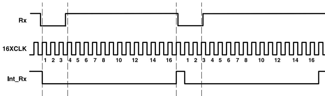
Figure 31. Timing Causing 1-Clock-Wide Pulse Between Consecutive Ones
