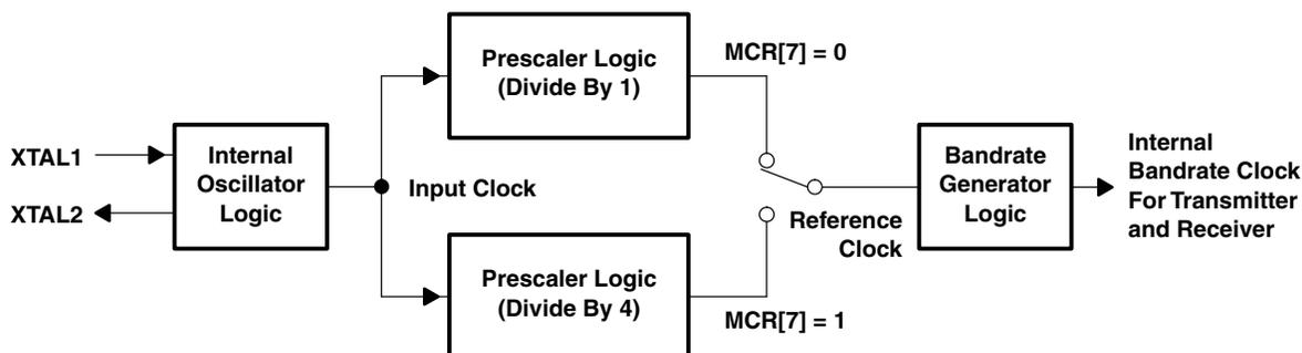
Figure 7. Prescaler and Baud Rate Generator Block Diagram
