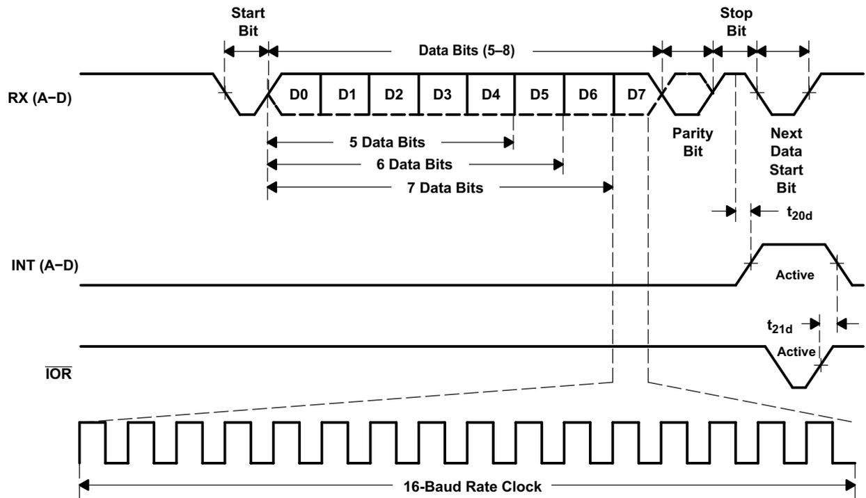
Figure 16. Receive Timing
