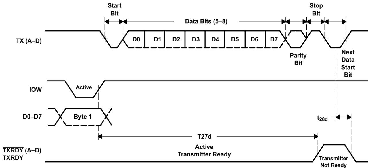
Figure 20. Transmit Ready Timing in None FIFO Mode
