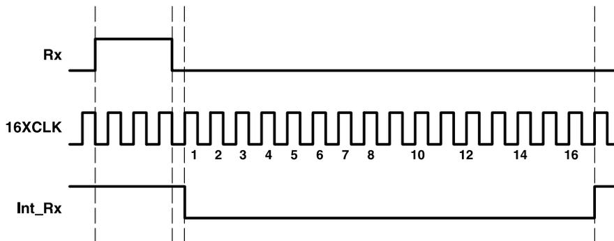
Figure 33. Positive Rx Pulse Decode – Detailed View
