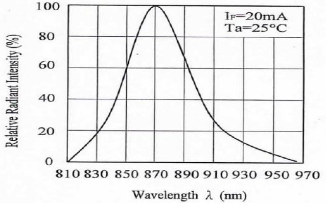
Fig.3 Peak Emission Wavelength Ambient Temperature
