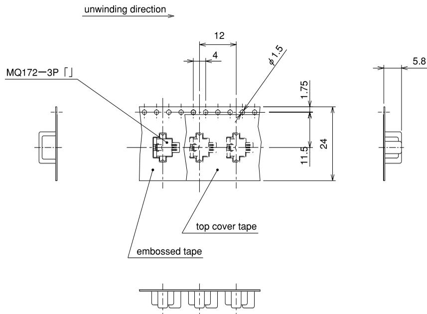
(Note.) The figure above provides the case of a 3 contact type, dimensions shown in such figure are the same as those of a 4 contact type.
