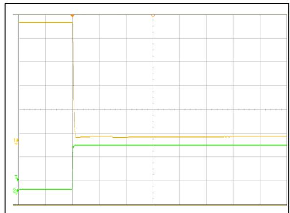
Figure 6: AVD85B-48S05 Remote OFF Waveform (10mS/div)
