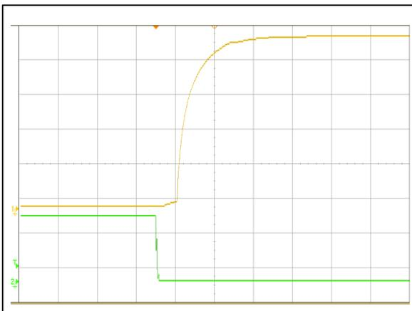
Figure 5: AVD85B-48S05 Remote ON Waveform (20mS/div)
