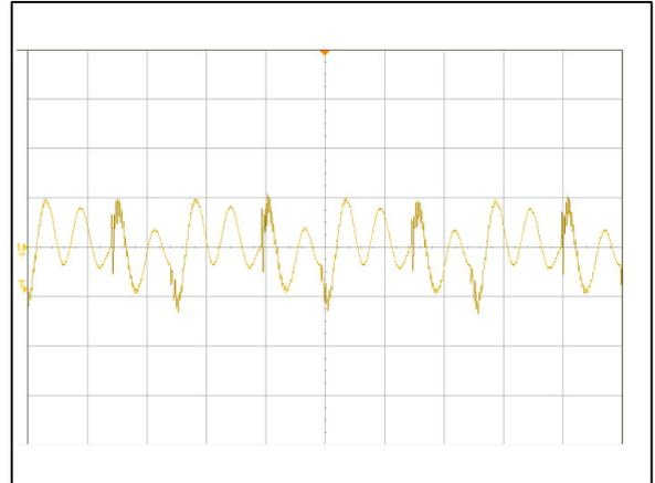
Figure 2: AVD85B-48S05 Ripple and Noise Measurement
