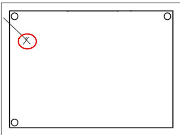
Figure 11: AVD50B-48S3V3B OTP test point (Module with baseplate)
