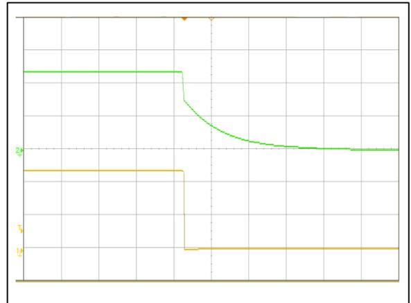
Figure 4: AVD85B-48S05 Turn Off Characteristic (20mS/div)
