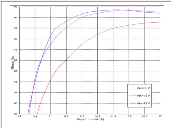
Figure 9: AVD85B-48S05 Efficiency Curves @ 25 °C, 400LFM
