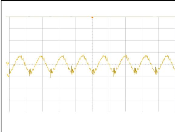
Figure 1: AVD85B-48S05 Input Reflected Ripple Current Waveform
