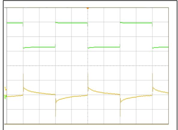
Figure 8: AVD85B-48S05 Transient Response (2mS/div)
