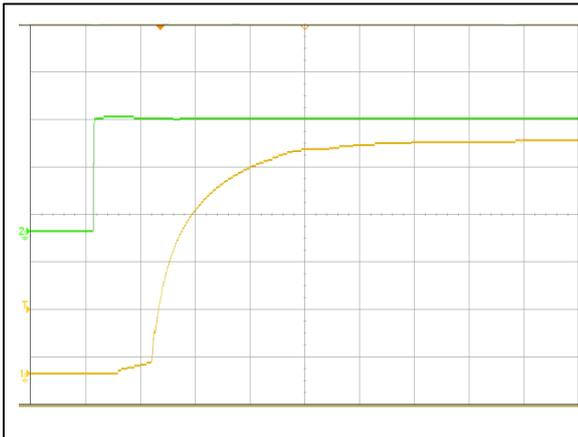
Figure 3: AVD85B-48S05 Output Voltage Startup Characteristic (10mS/div)
