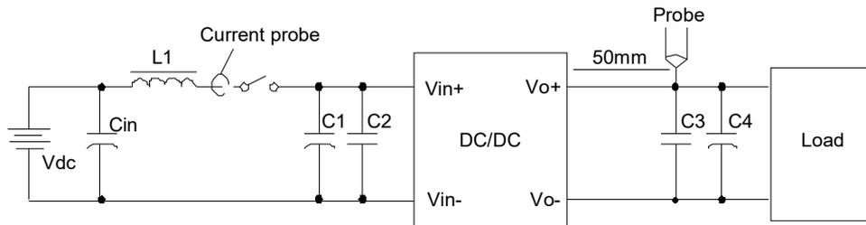
Figure 18 Input ripple & output ripple & noise test configuration
