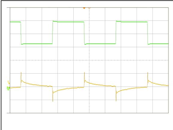
Figure 7: AVD85B-48S05 Transient Response (2mS/div)
