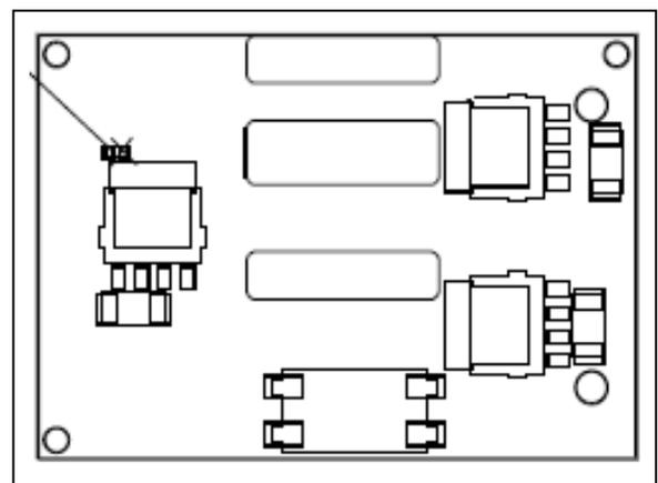
Figure 10: AVD50B-48S3V3 OTP test point (Open-frame module)
