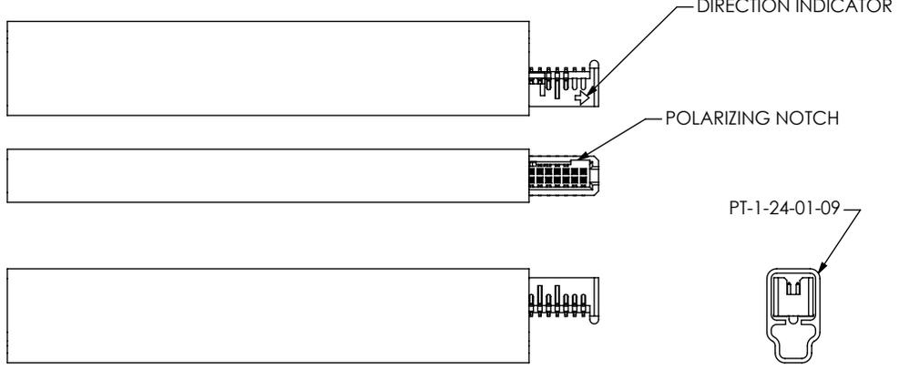
PARTS TO BE POSITIONED WITH TAILS FACING LOGO SIDE OF TUBE AND POLARIZING NOTCH ORIENTED AS SHOWN
