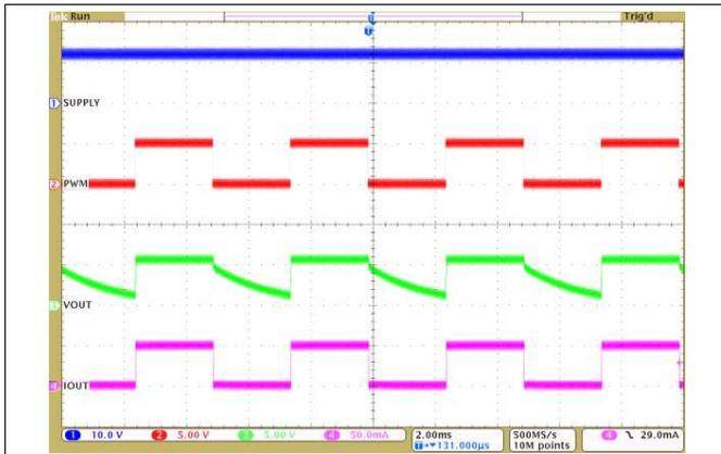
Ch. 1 =  $V_{(SUPPLY)}$  Ch. 2 =  $V_{(PWM)}$  Ch. 3 =  $I_{(OUT)}$
