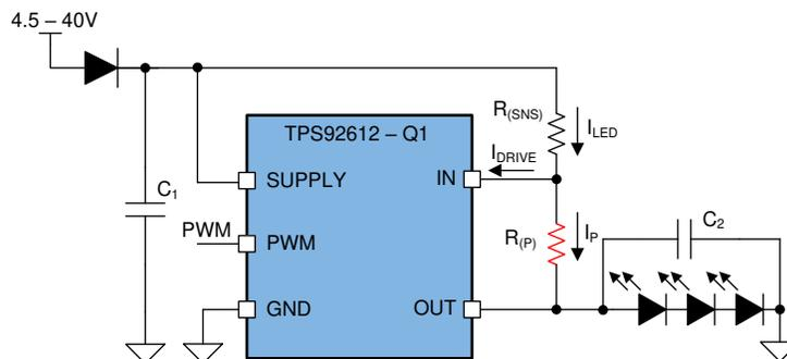
Figure 21. Heat Sharing With a Parallel Resistor
