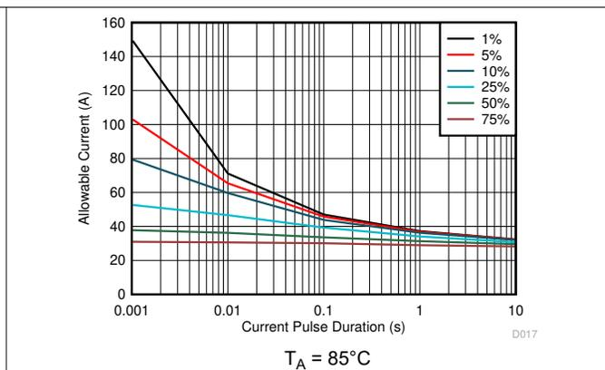
Figure 8-7. Maximum Repetitive Pulsed Current vs. Pulse Duration
