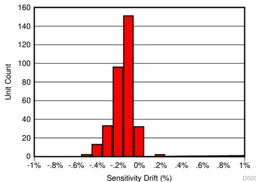
**Figure 9-4. Sensitivity Error After 130°C, 85% RH HAST**
