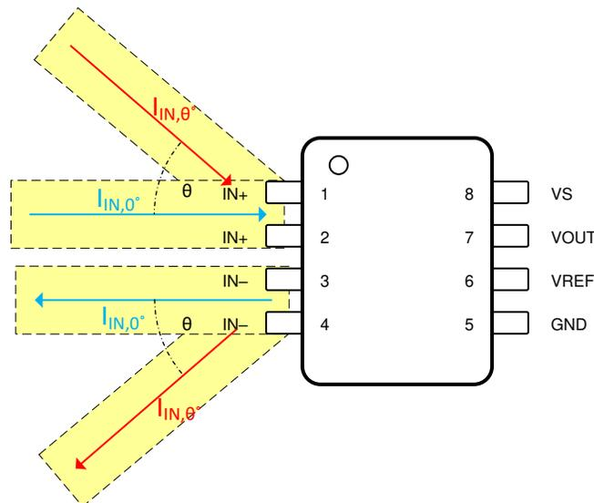
**Figure 12-1. Magnetic Field Generated by Input Current Trace**
