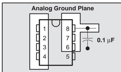
Figure 16. Power-Supply Bypassing
