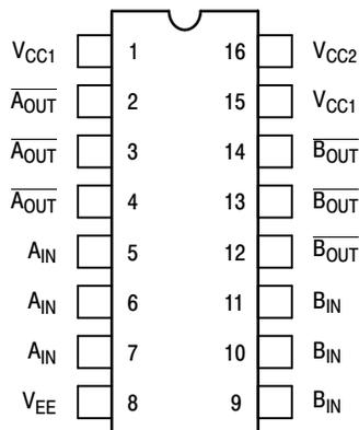
Pin assignment is for Dual-in-Line Package.
