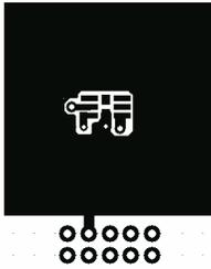
a)  $68^\circ\text{C}/\text{W}$  when mounted on a  $1\text{ in}^2$  pad of 2 oz copper (Single Operation).
