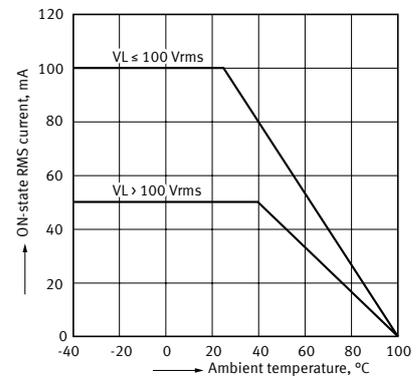
1-4.ON-state RMS current vs. ambient temperature characteristics
