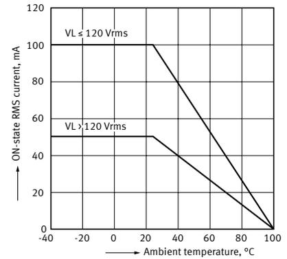
2. On voltage vs. ambient temperature characteristics
