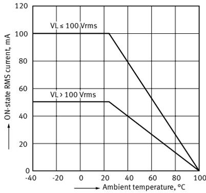
1-5.ON-state RMS current vs. ambient temperature characteristics
