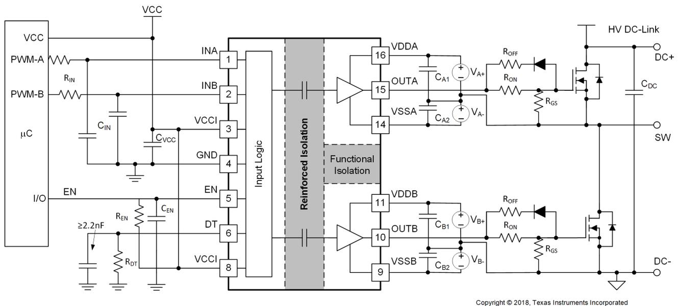
**Figure 9-1. Typical Application Schematic with Dual Power Supplies**
