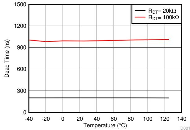
Figure 6-27. Dead Time vs. Temperature (with  $R_{DT} = 20\text{ k}\Omega$  and  $100\text{ k}\Omega$ )
