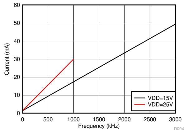
**Figure 6-5. Per Channel Current Consumption (I<sub>VDDA/B</sub>) vs. Frequency (1-nF Load, VDD = 15 V or 25 V)**
