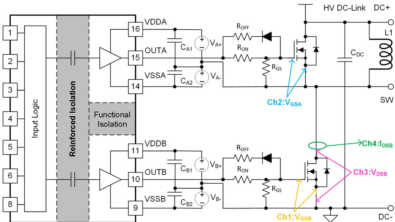
Figure 9-5. Bench Test Circuit with SiC MOSFET Switching
