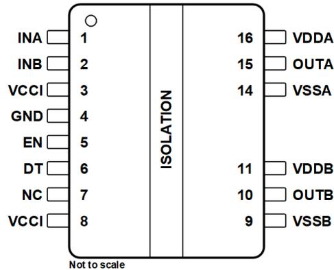
**Figure 5-1. DWK Package 14-Pin SOIC Top View**
