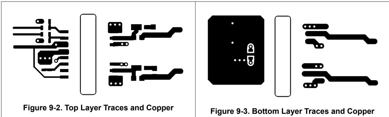
Figure 9-2. Top Layer Traces and Copper
