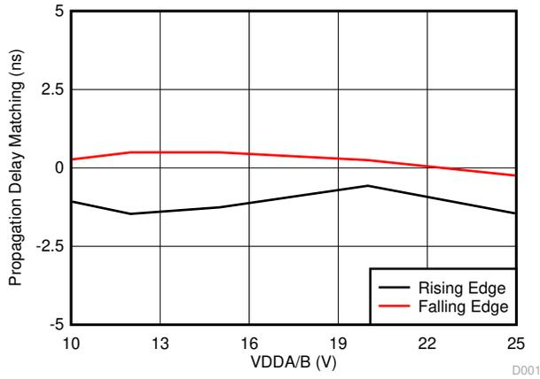
Figure 6-15. Propagation Delay Matching (t<sub>DM</sub>) vs. VDD
