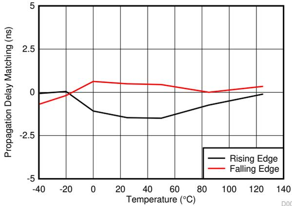
Figure 6-16. Propagation Delay Matching ( $t_{DM}$ ) vs. Temperature
