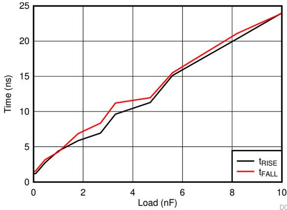
Figure 6-10. Rising and Falling Times vs. Load
