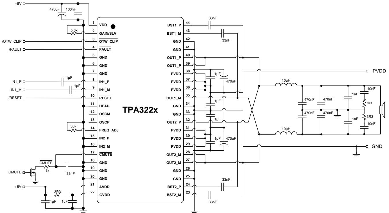
Figure 51. Typical Differential (2N) AD-Mode PBTL Application
