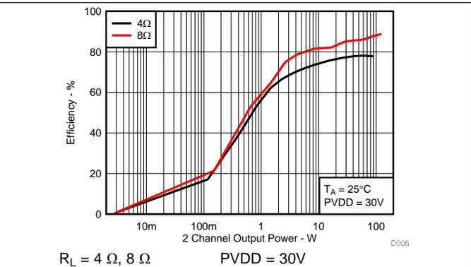
Figure 6. System Efficiency vs Output Power, AD-mode
