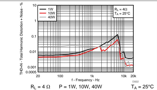
Figure 2. Total Harmonic Distortion+Noise vs Frequency, AD-mode
