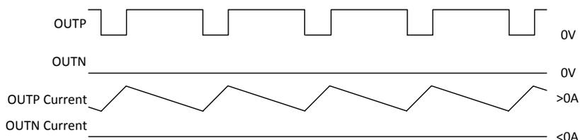
Figure 40. HEAD Mode Output Waveforms, High Level Output
