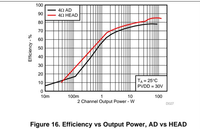
**Figure 16. Efficiency vs Output Power, AD vs HEAD**
