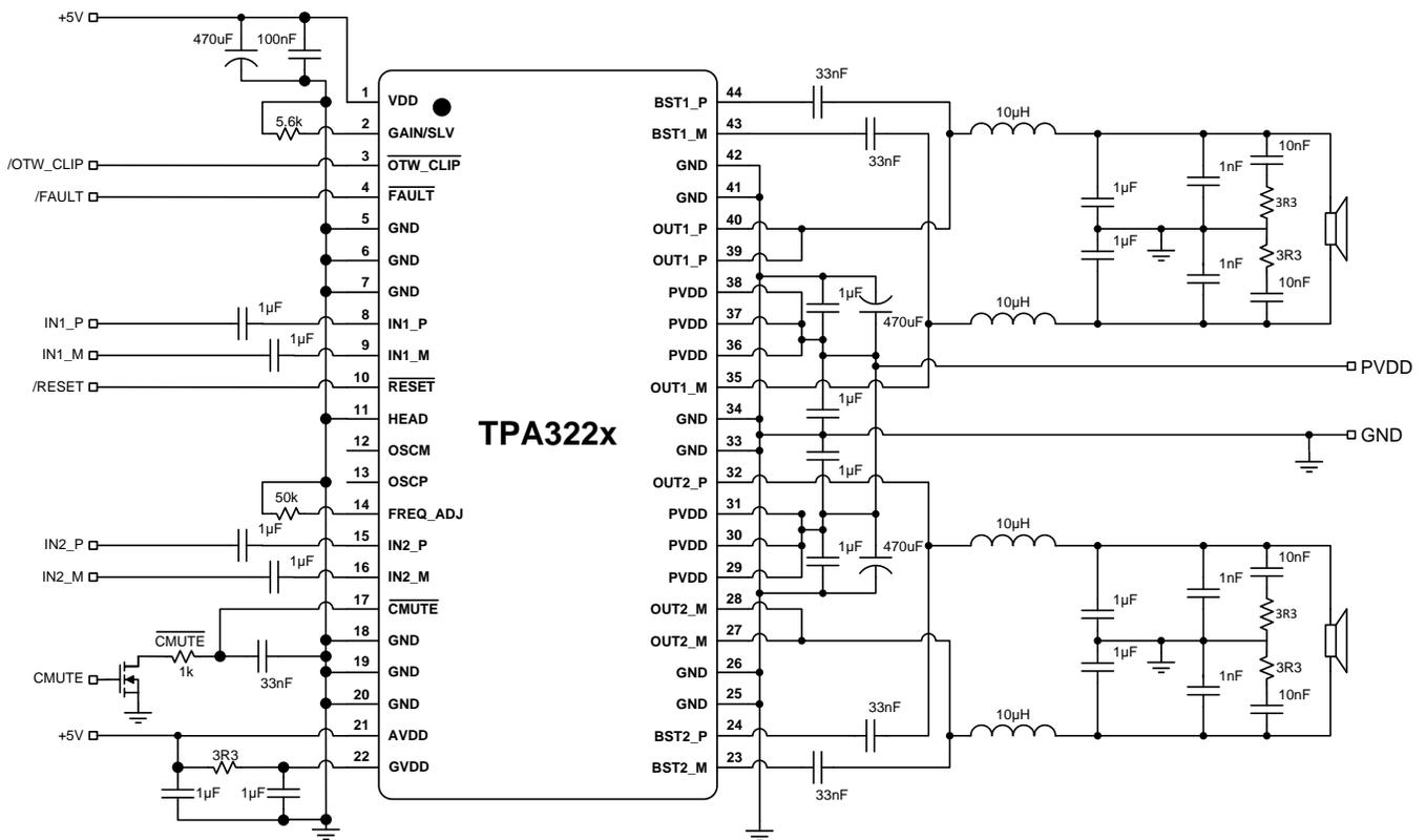
Figure 50. Typical Differential (2N) AD-Mode BTL Application
