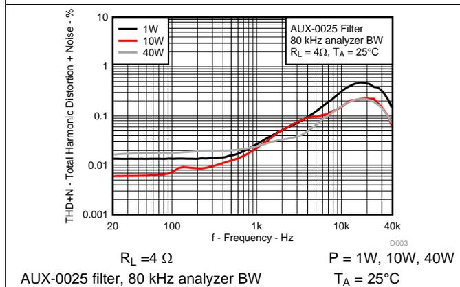
Figure 3. Total Harmonic Distortion+Noise vs Frequency, AD-mode
