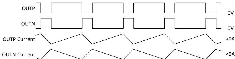
Figure 37. AD Mode Output Waveforms, High Level Output
