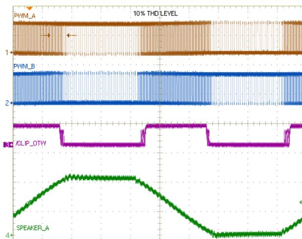
Figure 49. Signal Clipping PWM and Speaker Output Signals
