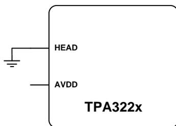
Figure 34. AD-Mode Configuration
