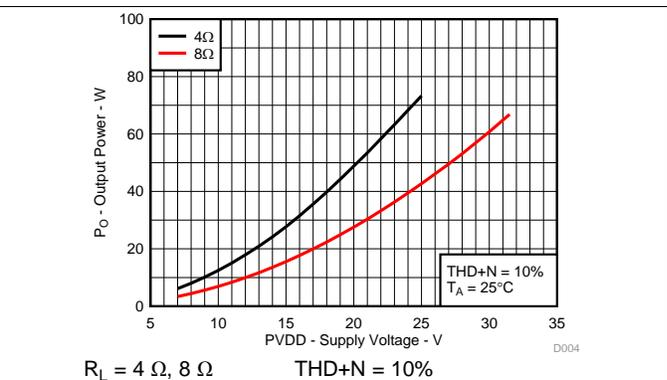
Figure 4. Output Power vs Supply Voltage, AD-mode
