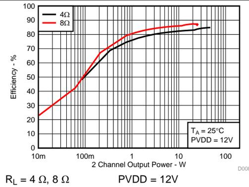
Figure 8. System Efficiency vs Output Power, AD-mode
