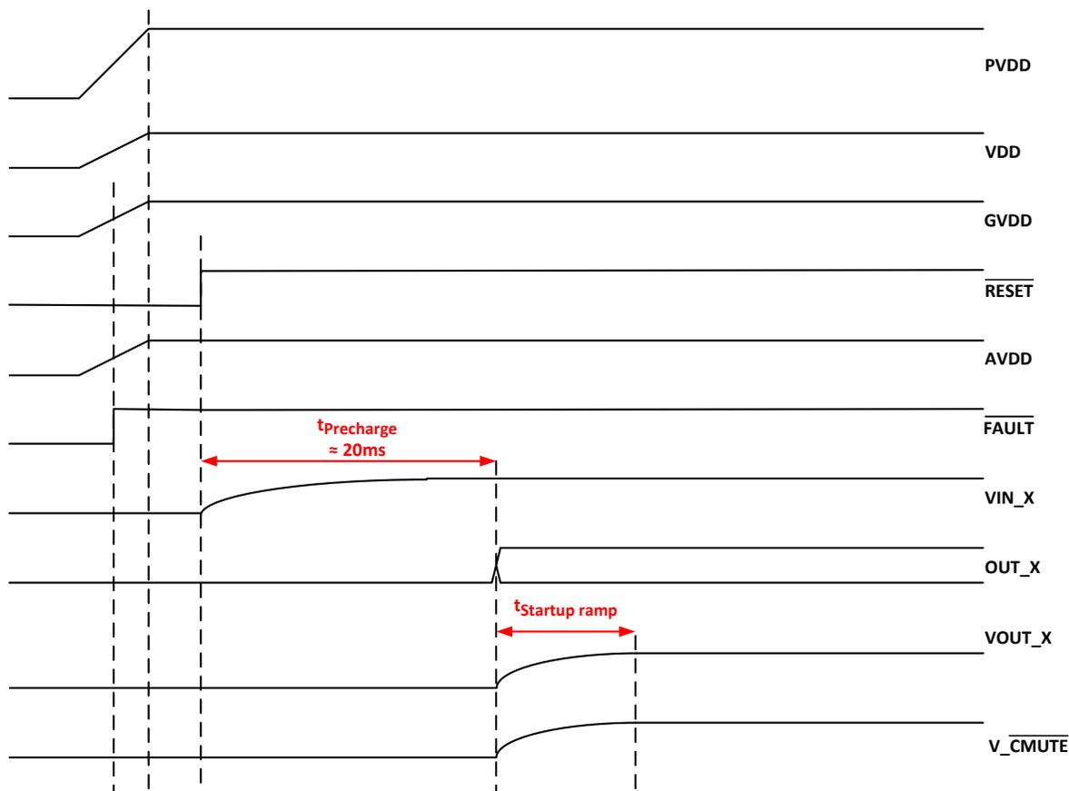
Figure 47. Startup Timing
