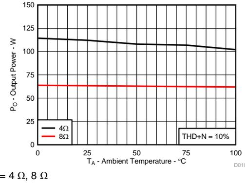
Figure 10. Output Power vs Ambient Temperature, AD-mode
