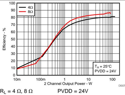
Figure 7. System Efficiency vs Output Power, AD-mode
