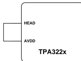
Figure 35. HEAD-Mode Configuration
