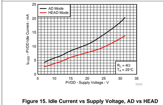
**Figure 15. Idle Current vs Supply Voltage, AD vs HEAD**
