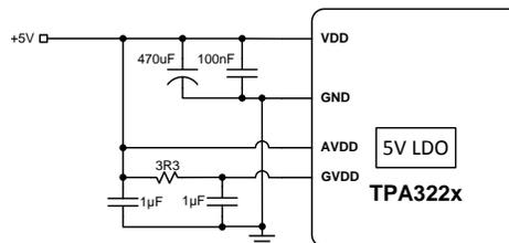
Figure 29. Internal LDO Bypass for Highest Power Efficiency
