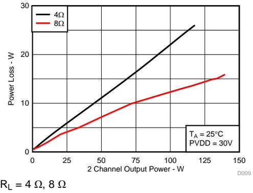
Figure 9. System Power Loss vs Output Power, AD-mode
