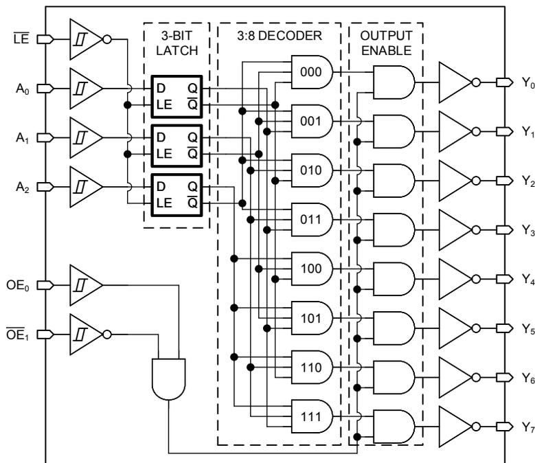
Figure 8-1. Logic Diagram (Positive Logic) for the SN74HCS137-Q1
