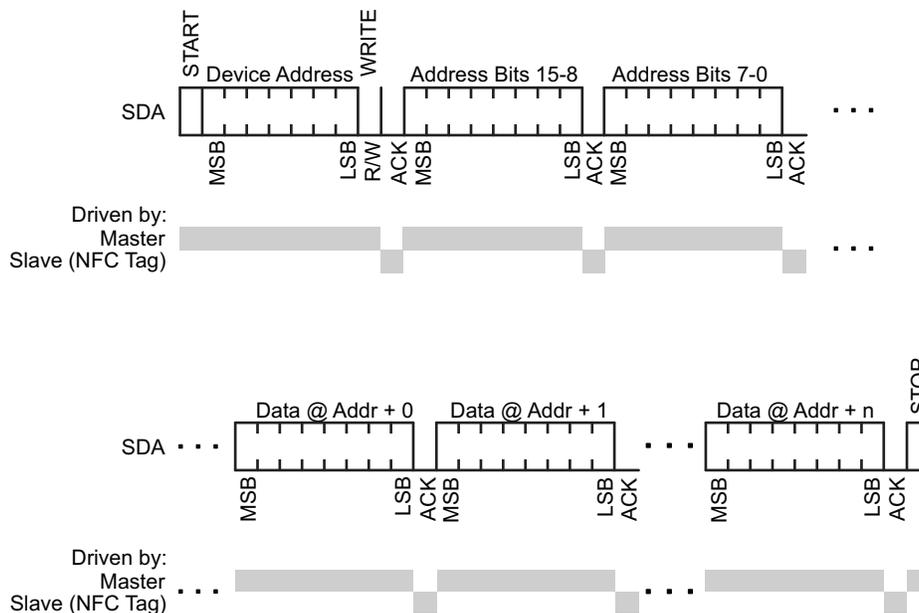
**Figure 5-2. I<sup>2</sup>C Write Access**
