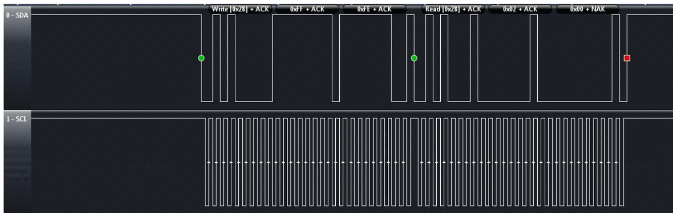
Figure 5-5. I<sup>2</sup>C Access Example: Read of the Control Register at Address 0xFFFE, Responds With 0x00, 0x02 (RF Enable = 1)
