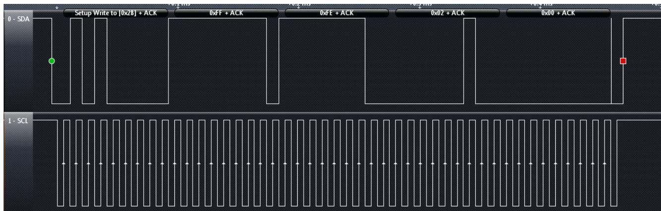
Figure 5-4. I<sup>2</sup>C Access Example: Write of the Control Register at Address 0xFFFE With 0x00, 0x02 (RF Enable = 1)
