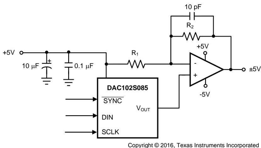
**Figure 37. Bipolar Operation**
