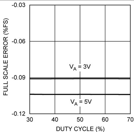
Figure 23. Full-Scale Error vs Clock Duty Cycle
