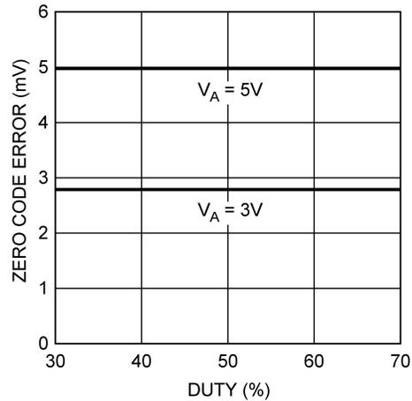
Figure 18. Zero Code Error vs Clock Duty Cycle
