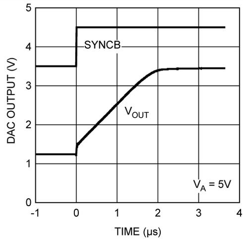
**Figure 21. Settling Time**
