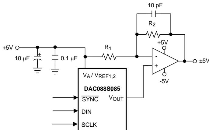
Figure 32. Bipolar Operation
