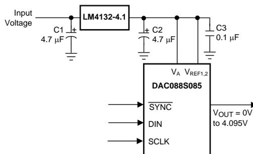
Figure 43. The LM4132 as a Power Supply
