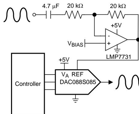
Figure 41. Programmable Attenuator Diagram
