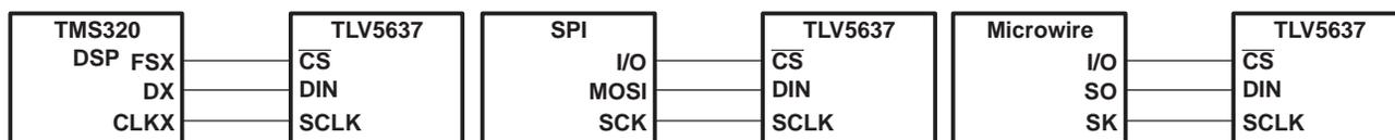
**Figure 13. Three-Wire Interface**
