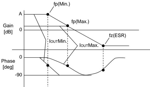
Fig.38 Open loop gain characteristics
