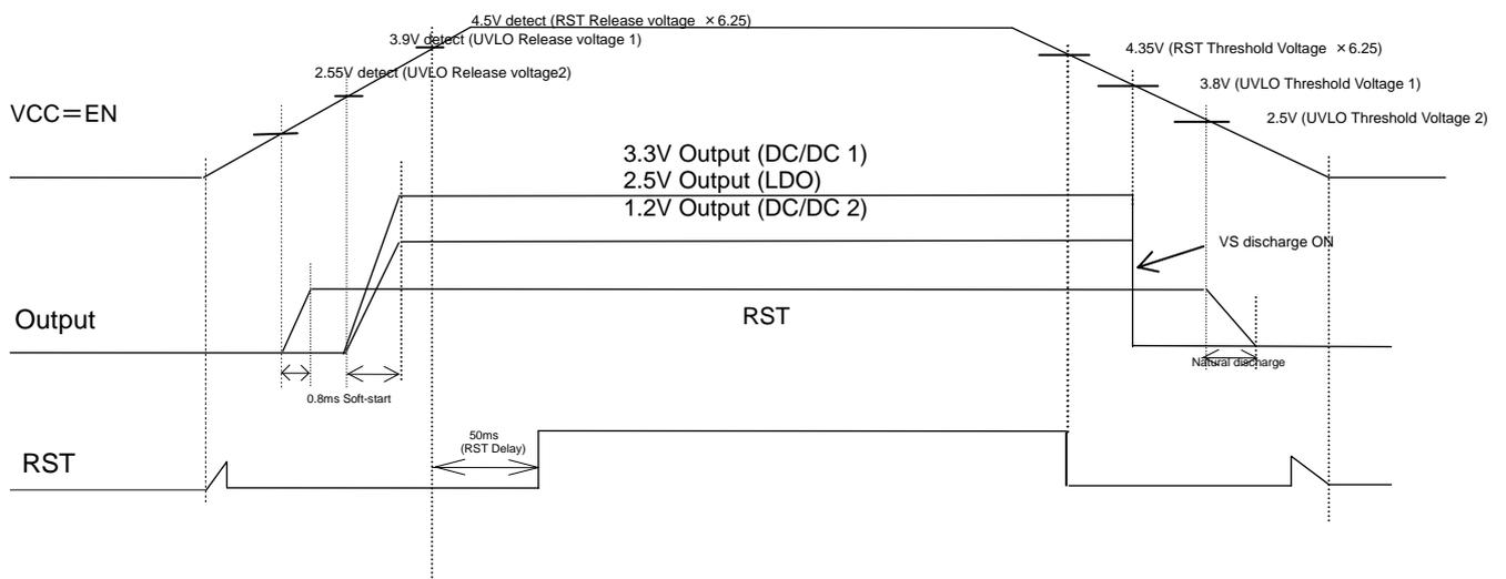
Fig.32 Soft-start, Shutdown, RST Delay, UVLO, timing chart
