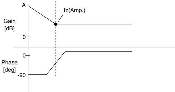
Fig.39 Error amp phase compensation characteristics
