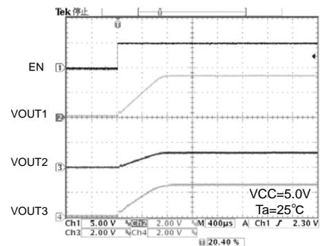
Fig.14 Soft start wave form (Io<sub>1</sub>=0mA, Io<sub>2</sub>=0mA, Io<sub>3</sub>=0mA)
