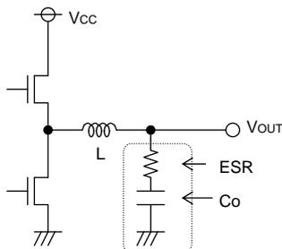
Fig.36 Output capacitor
