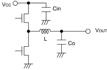
Fig.37 Input capacitor
