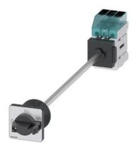
Load disconnector 3LD3, lu 40 A Main switch 3-pole Rated operating capacity at AC-23 A at 400 V 18.5 kW floor mounting Basic switch with door coupling Central hole mounting 22.5mm Toggle drive black 48x48 mm
