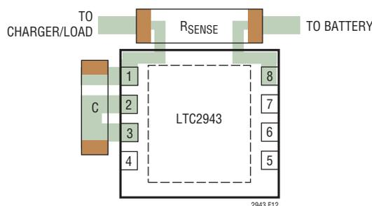
Figure 12. Kelvin Connection on Sense Resistor
