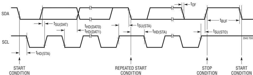
Figure 1. Definition of Timing on I<sup>2</sup>C Bus
