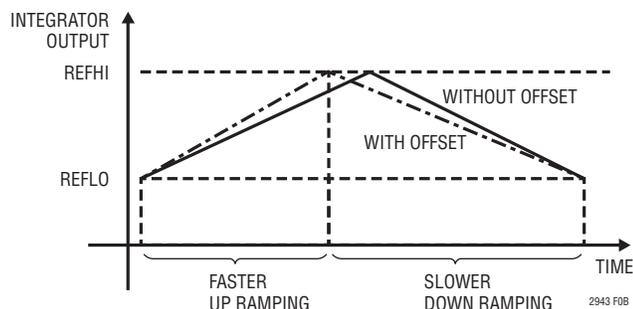
For input signals with an absolute value smaller than the offset of the internal op amp, the LTC2943 stops integrating and does not integrate its own offset.
