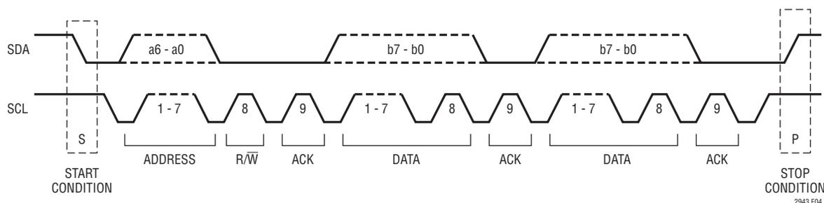
Figure 4. Data Transfer Over I<sup>2</sup>C or SMBus
