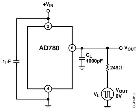
Figure 18. Capacitive Load Transient Response Test Circuit
