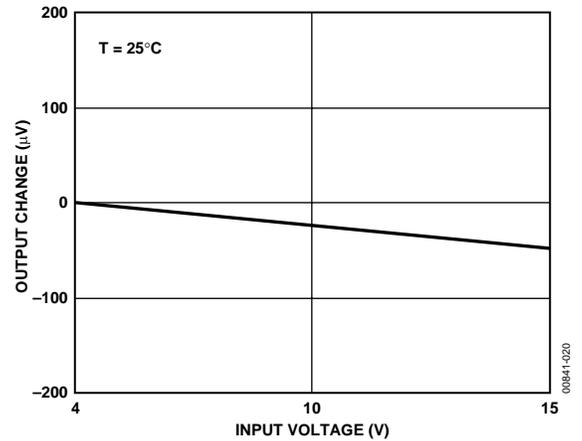
Figure 20. Output Voltage Change vs. Input Voltage
