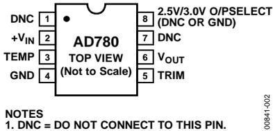
Figure 2. Pin Configuration, 8-Lead PDIP and SOIC Packages
