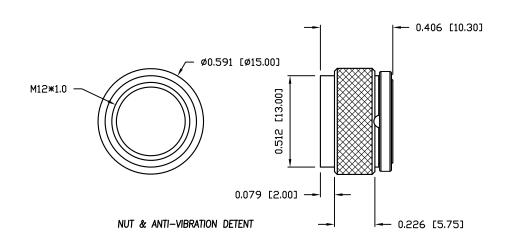
NΠΤF: MATERIAL HOUSING: PA66 UL94V-0, BLACK CONTACT: **BRASS** NUT: **BRASS** □-RING: EPDM, BLACK FINISH 10u" GOLD PLATED CONTACT: **NICKEL** NUT: **ELECTRICAL** RATED CURRENT: 4A RATED VOLTAGE: 60V INSULATOR RESISTANCE: 100 MOhms MIN. CONTACT RESISTANCE: 10 mOhms MAX.
