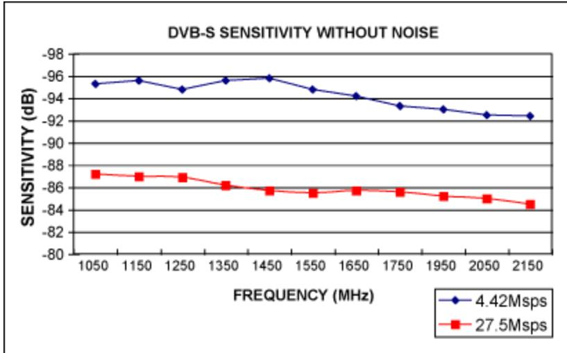
Figure 3. The DVB-S sensitivity without noise is better than -92.5dBm for 4.42Mps, and better than -84dBm for 27.5Mps across the band.
