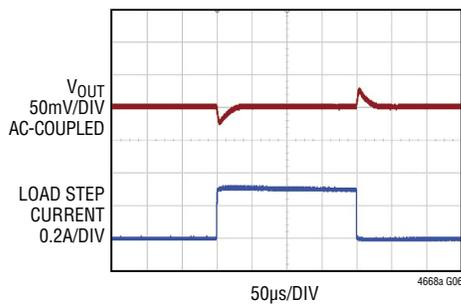
V<sub>IN</sub> = 12V, V<sub>OUT</sub> = 1.8V, f<sub>S</sub> = 2.25MHz
