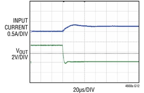
$V_{IN} = 12V$ ,  $V_{OUT} = 3.3V$ ,  $f_S = 2.25MHz$
