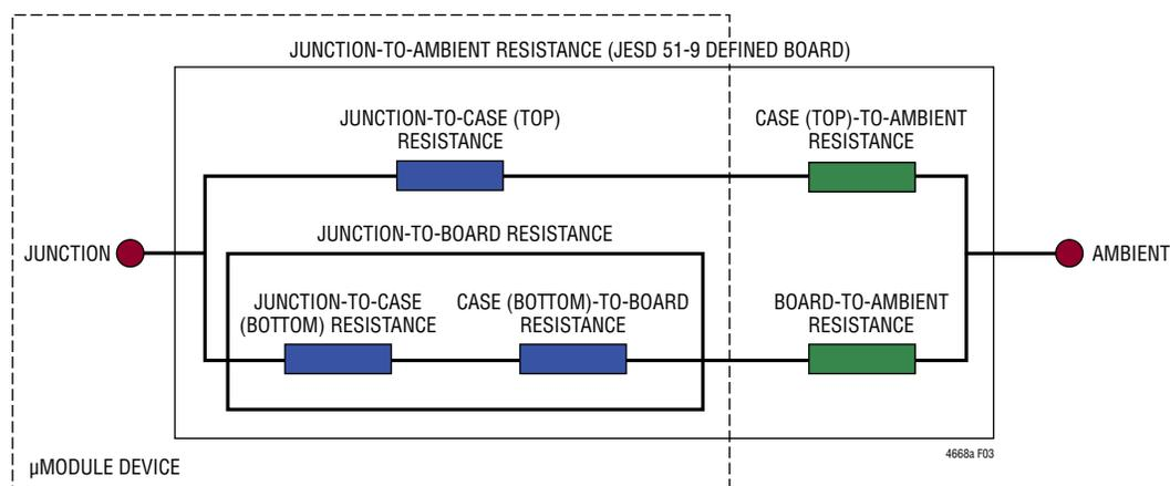
Figure 3. Graphical Representation of JESD51-12 Thermal Coefficients
