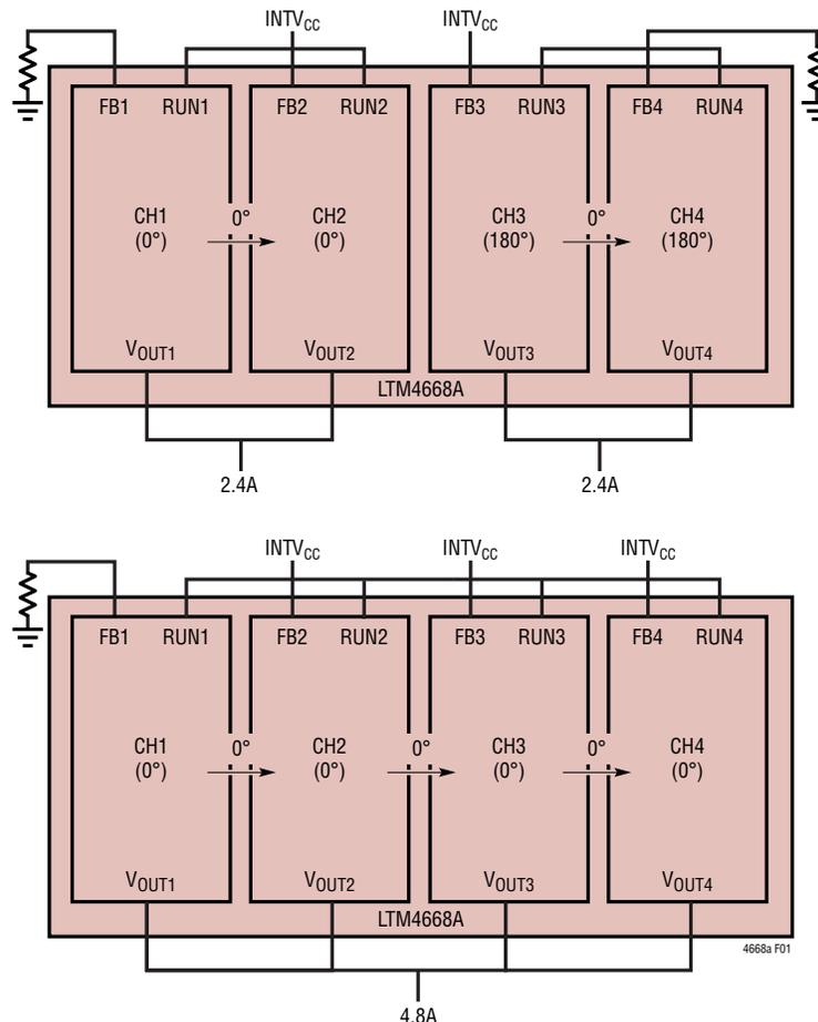
**Figure 1. 2+2 and 4-Channel Parallel Concept Schematic**
