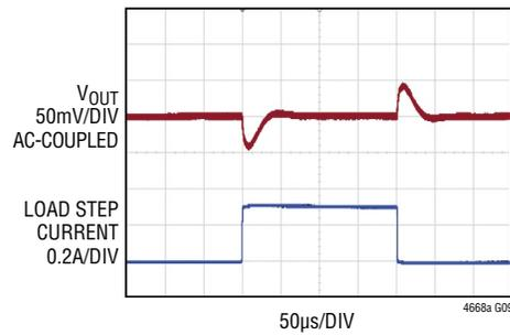
V<sub>IN</sub> = 12V, V<sub>OUT</sub> = 5V, f<sub>S</sub> = 2.25MHz
