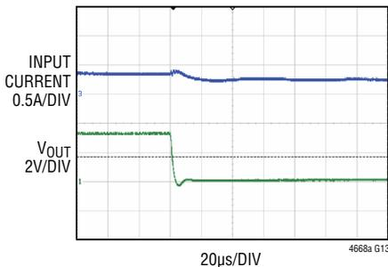
$V_{IN} = 12V$ ,  $V_{OUT} = 3.3V$ ,  $f_S = 2.25MHz$
