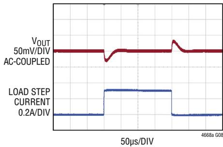
V<sub>IN</sub> = 12V, V<sub>OUT</sub> = 3.3V, f<sub>S</sub> = 2.25MHz
