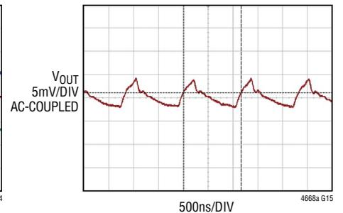
$V_{IN} = 12V$ ,  $V_{OUT} = 3.3V$ ,  $f_S = 2.25MHz$
