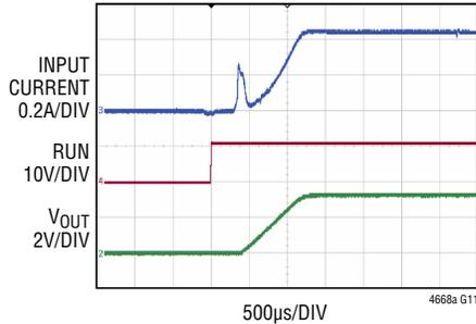
$V_{IN} = 12V$ ,  $V_{OUT} = 3.3V$ ,  $f_S = 2.25MHz$
