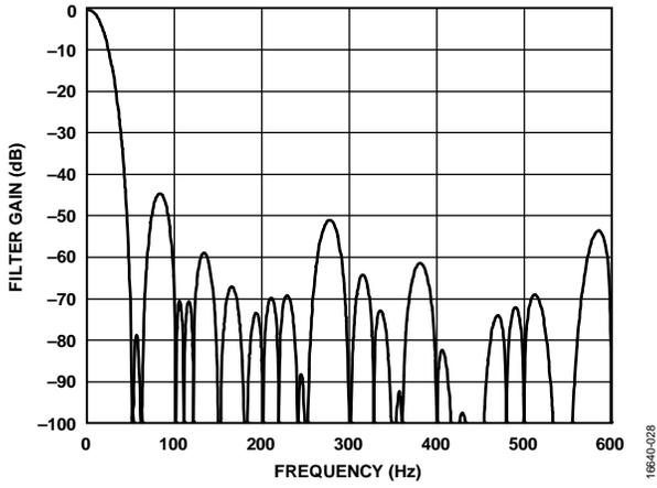
Figure 52. 16.667 SPS ODR, 60 ms Settling Time
