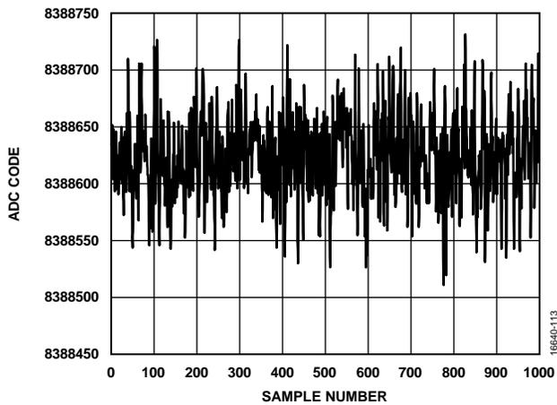
Figure 13. Noise (Current Input, Output Data Rate = 31.25 kSPS)
