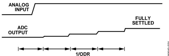
Figure 44. Step Input Without Single Cycle Settling
