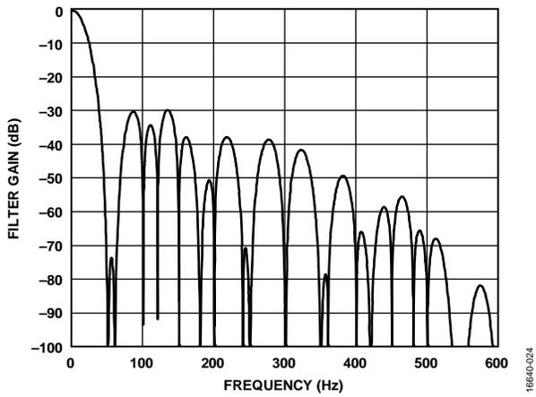
Figure 48. 20 SPS ODR, 50 ms Settling Time
