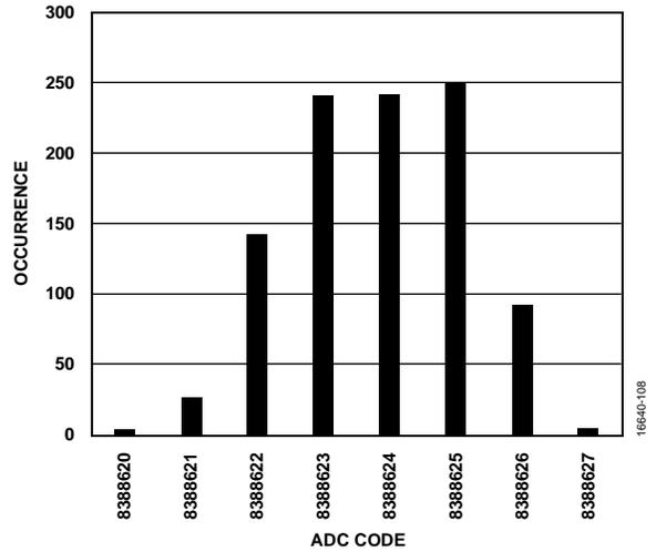
Figure 8. Histogram (Voltage Input, Output Data Rate = 1.25 SPS)
