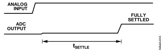
Figure 45. Step Input with Single Cycle Settling
