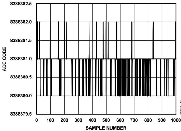
Figure 11. Noise (Current Input, Output Data Rate = 1.25 SPS)
