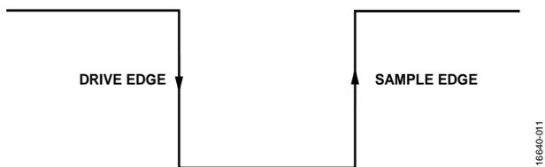
Figure 32. SPI Mode 3 SCLK Edges
