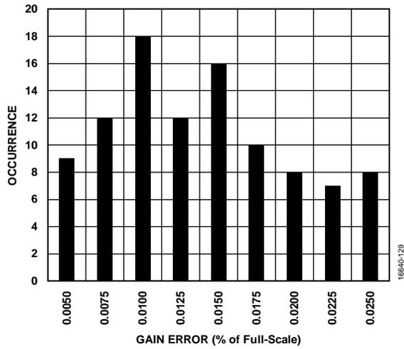
Figure 29. Gain Error Distribution Histogram (Current Input)
