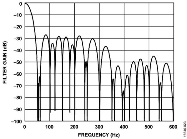
Figure 47. 25 SPS ODR, 40 ms Settling Time
