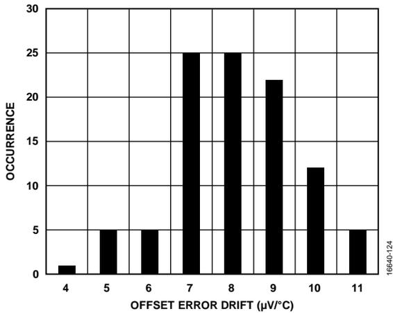
Figure 24. Offset Error Drift Distribution Histogram (Voltage Input)
