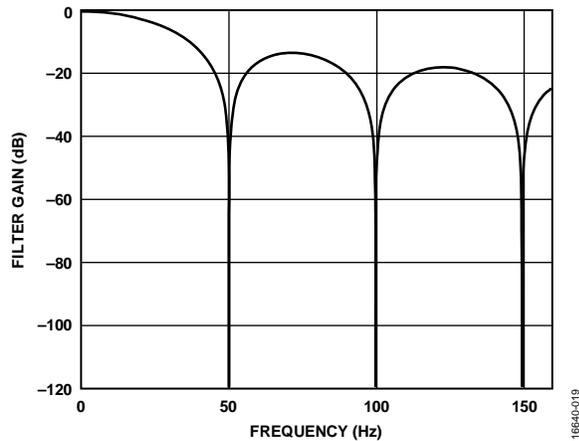
Figure 42. Sinc5 + Sinc1 Filter Response at 50 SPS ODR
