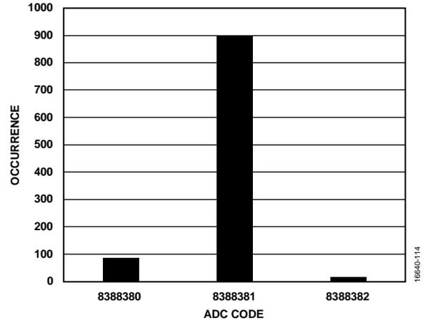
Figure 14. Histogram (Current Input, Output Data Rate = 1.25 SPS)
