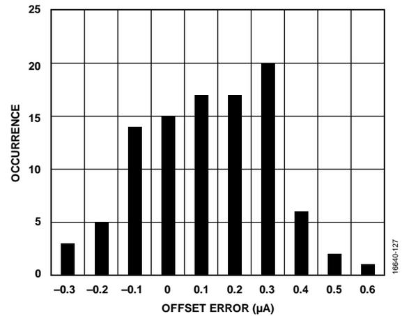
Figure 27. Offset Error Distribution Histogram (Current Input)
