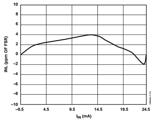
Figure 19. Integral Nonlinearity (INL) vs. Input (Current Input)
