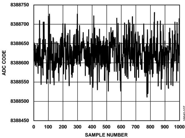
Figure 7. Noise (Voltage Input, Output Data Rate = 31.25 kSPS)
