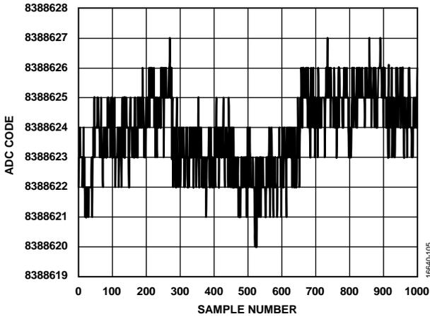
Figure 5. Noise (Voltage Input, Output Data Rate = 1.25 SPS)
