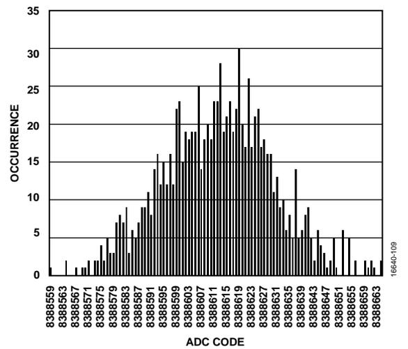
Figure 9. Histogram (Voltage Input, Output Data Rate = 2.5 kSPS)
