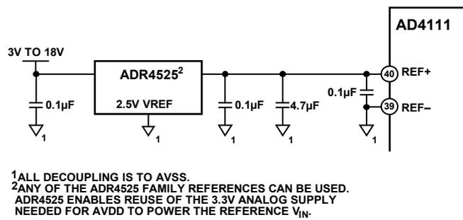
Figure 39. ADR4525 Connected to AD4111 REF± Pins
