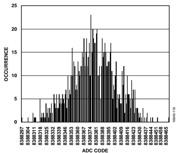
Figure 16. Histogram (Current Input, Output Data Rate = 31.25 kSPS)
