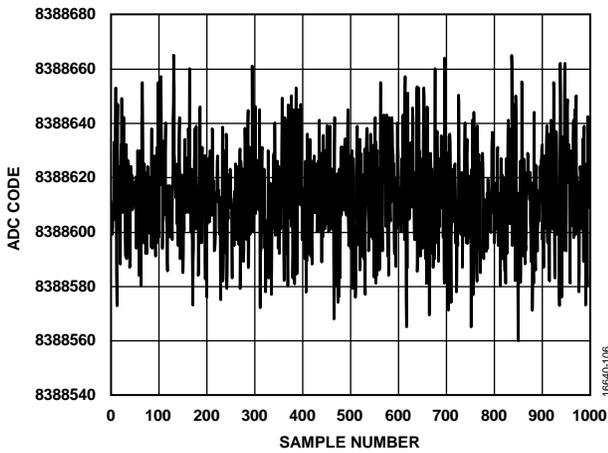
Figure 6. Noise (Voltage Input, Output Data Rate = 2.5 kSPS)
