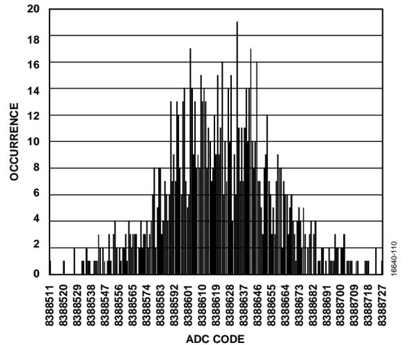
Figure 10. Histogram (Voltage Input, Output Data Rate = 31.25 kSPS)
