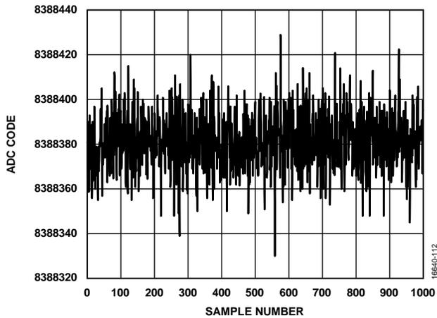
Figure 12. Noise (Current Input, Output Data Rate = 2.5 kSPS)
