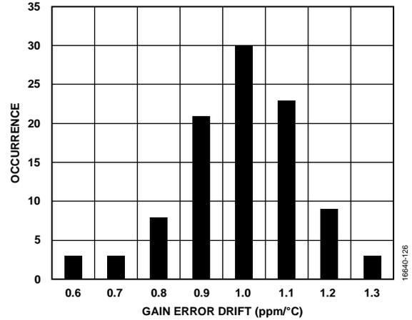
Figure 26. Gain Error Drift Distribution Histogram (Voltage Input)
