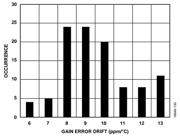
Figure 30. Gain Error Drift Distribution Histogram (Current Input)
