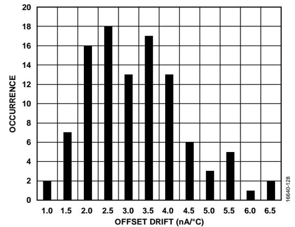
Figure 28. Offset Error Drift Distribution Histogram (Current Input)
