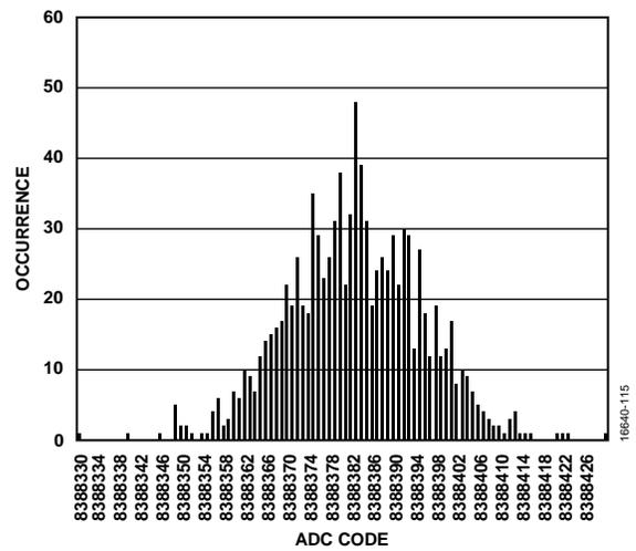
Figure 15. Histogram (Current Input, Output Data Rate = 31.25 SPS)
