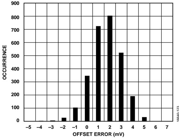
Figure 23. Offset Error Distribution Histogram (Voltage Input)
