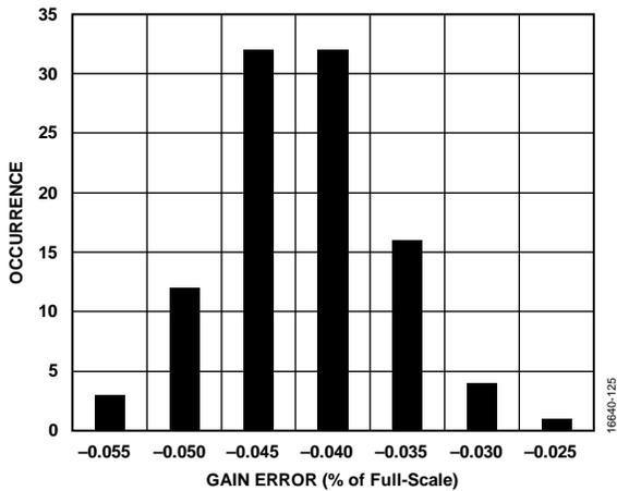
Figure 25. Gain Error Distribution Histogram (Voltage Input)
