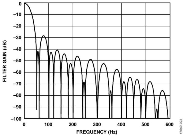
Figure 46. 27.27 SPS ODR, 36.67 ms Settling Time
