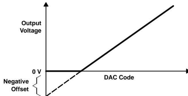
**Figure 13. Effect of Negative Offset (Single Supply)**
