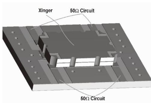
**Figure 3: Component Placement**
