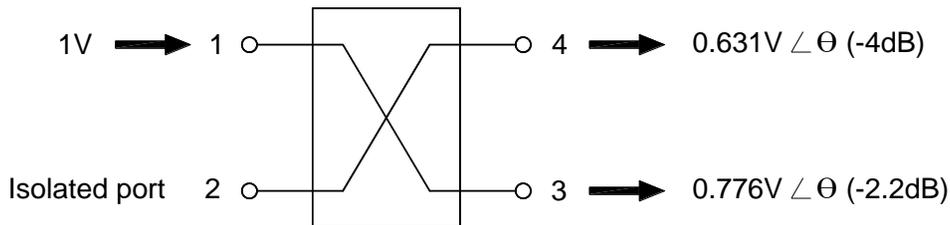
The primary application for 4dB couplers is in serial splitting and combining networks. These networks are often employed when the combining of 3 amplifiers is required. Unlike corporate networks, serial networks are not limited to binary divisions (corporate networks are limited to  $2^n$  number of splits, where  $n$  is an integer). Serial networks can be designed with [3, 4, 5, ...,  $n$ ] splits, but have a practical limitation of about 8 splits.
