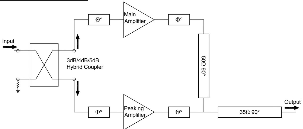
Hybrid coupler can be used in Doherty power amplifier to split the input power into the desired power ratio and phase delay. In above symmetrical Doherty power amplifier (main and peaking amplifier delivers equal amount output power at max drive condition), 3dB hybrid splits the input power into 1:1 ratio with 90 degree phase difference.
