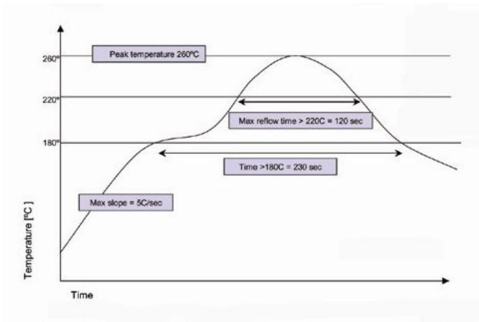
Figure 6 – High Temperature Solder Reflow Thermal Profile
