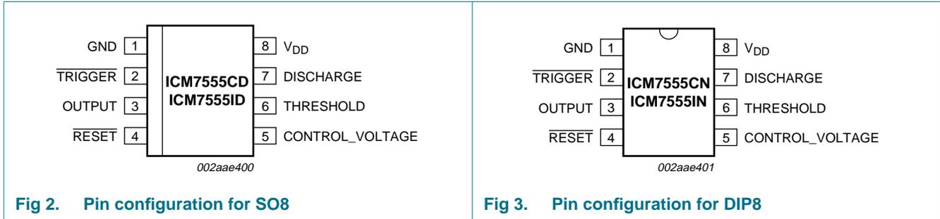
Fig 2. Pin configuration for SO8
