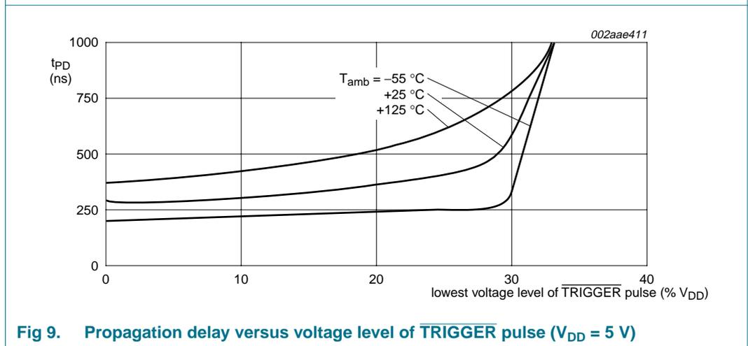
Fig 9. Propagation delay versus voltage level of TRIGGER pulse ( $V_{DD} = 5\text{ V}$ )
