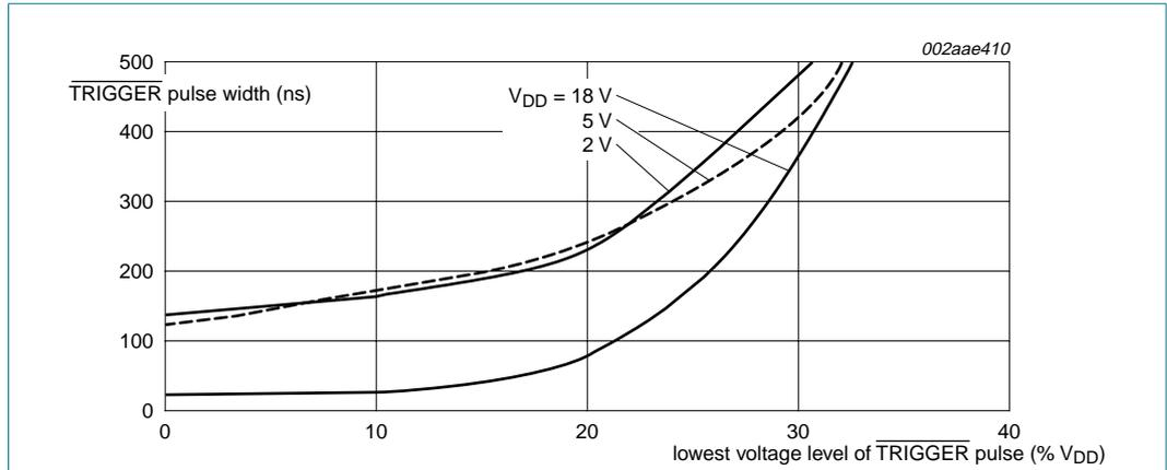
Fig 8. Minimum pulse width for triggering
