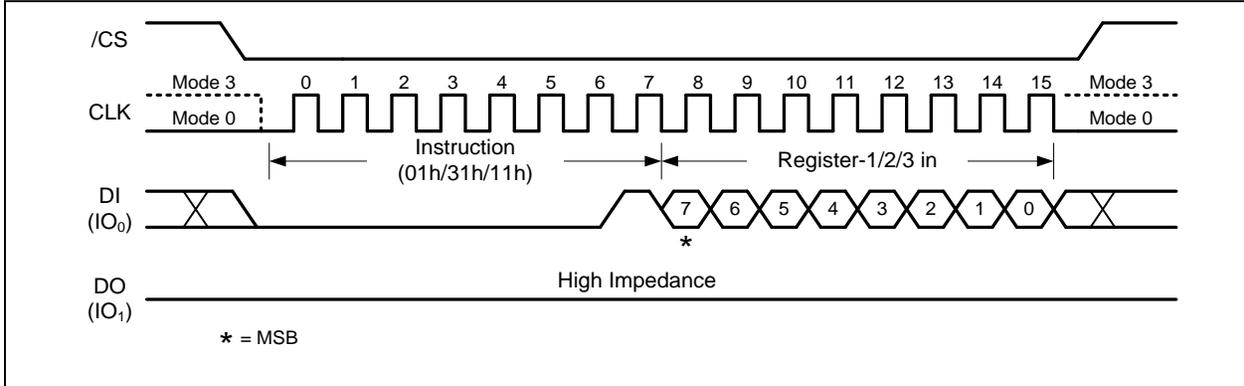
Figure 9a. Write Status Register-1/2/3 Instruction (SPI Mode)
