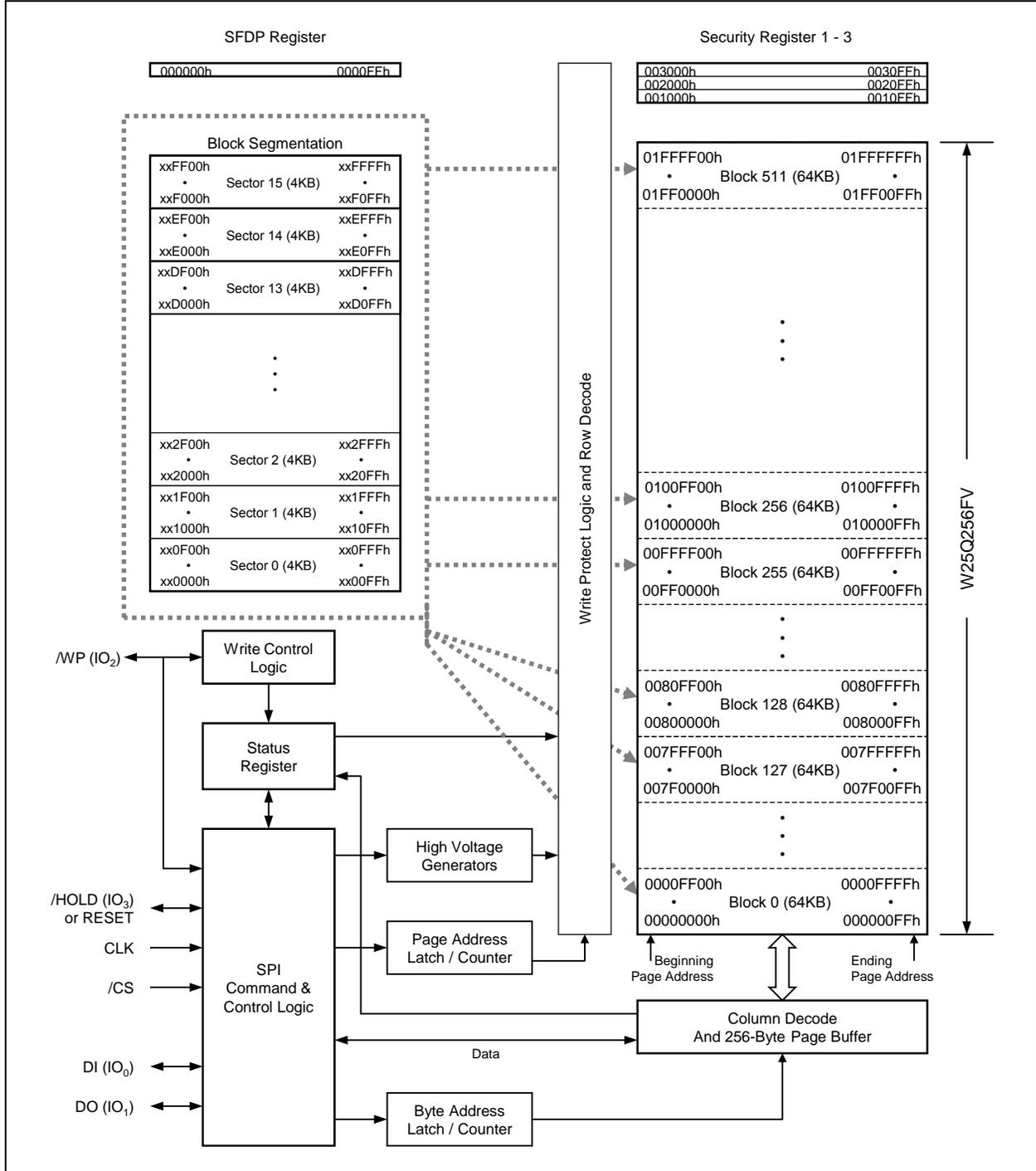
Figure 2. W25Q256FV Serial Flash Memory Block Diagram
