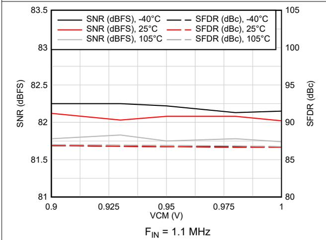
**Figure 6-11. AC Performance vs VCM vs Temperature**
