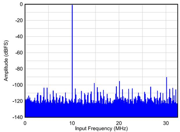
**Figure 6-43. Single Tone FFT at  $F_{IN} = 10\text{ MHz}$**
