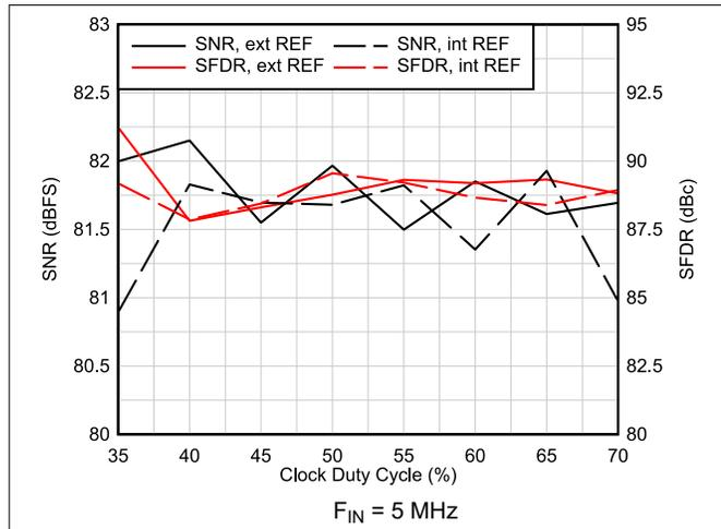
Figure 6-58. AC Performance vs Clock Duty Cycle
