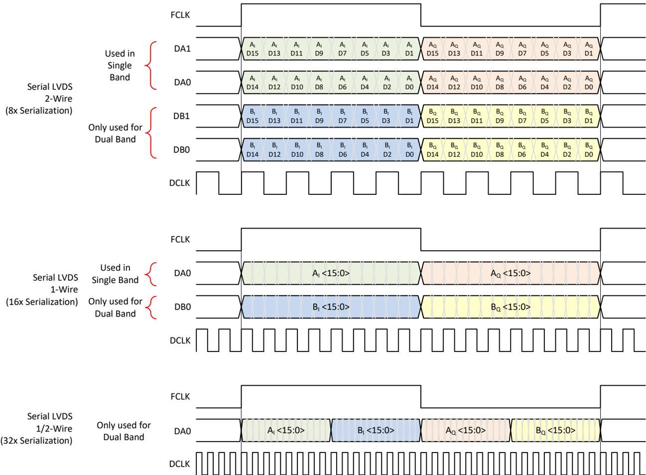
**Figure 8-39. Output Data Format in Complex Decimation**
