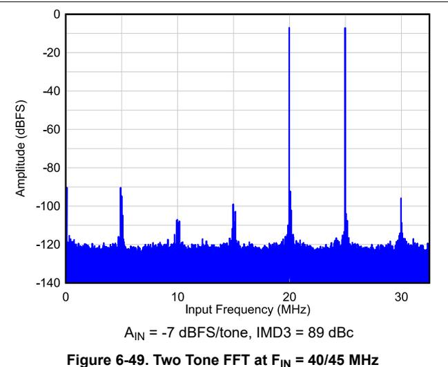
Figure 6-49. Two Tone FFT at  $F_{IN} = 40/45\text{ MHz}$
