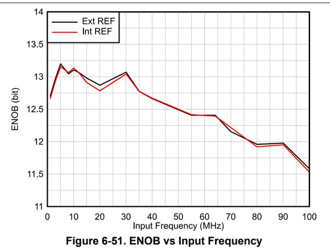
Figure 6-51. ENOB vs Input Frequency
