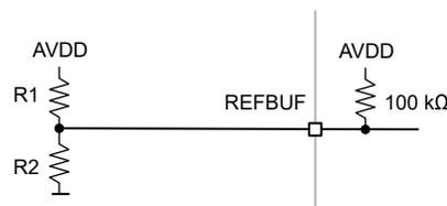
**Figure 8-51. Configuration of external voltage on REFBUF pin**
