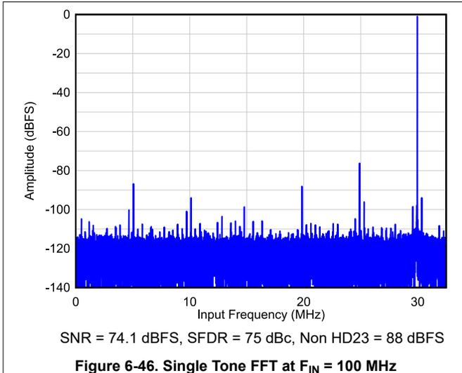
Figure 6-46. Single Tone FFT at  $F_{IN} = 100\text{ MHz}$
