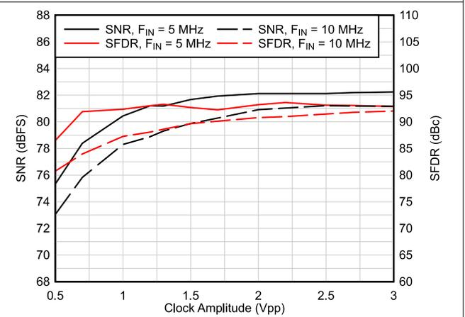
Figure 6-55. AC Performance vs Clock Amplitude
