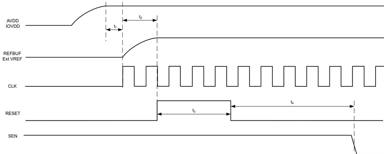
**Figure 9-6. Initialization of serial registers after power up**
