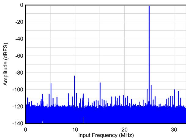
**Figure 6-44. Single Tone FFT at  $F_{IN} = 40\text{ MHz}$**
