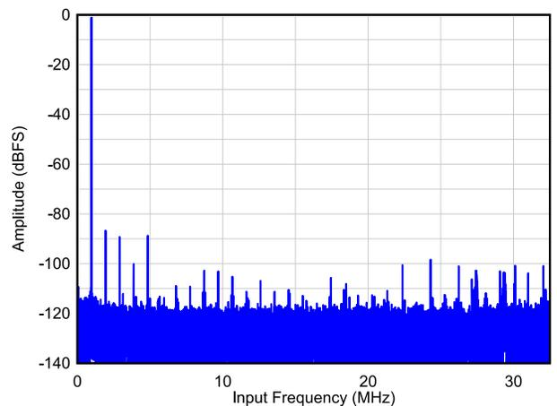
**Figure 6-45. Single Tone FFT at  $F_{IN} = 64\text{ MHz}$**
