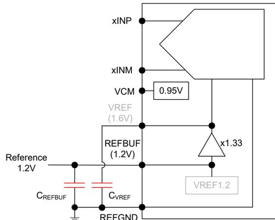
**Figure 8-20. External 1.2V reference using internal reference buffer**
