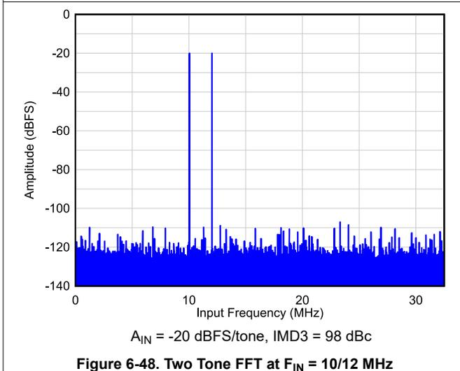
Figure 6-48. Two Tone FFT at  $F_{IN} = 10/12\text{ MHz}$
