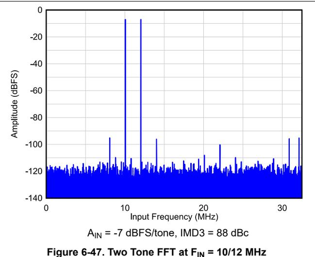
Figure 6-47. Two Tone FFT at  $F_{IN} = 10/12\text{ MHz}$
