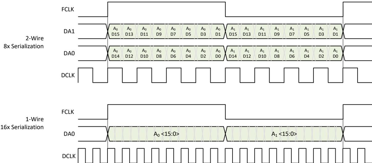
Figure 8-40. Output Data Format in Real Decimation
