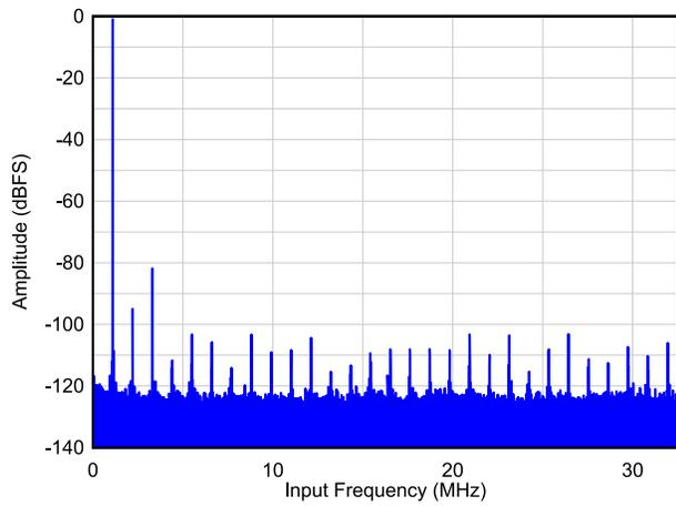
**Figure 6-40. Single Tone FFT at  $F_{IN} = 1\text{ MHz}$**
