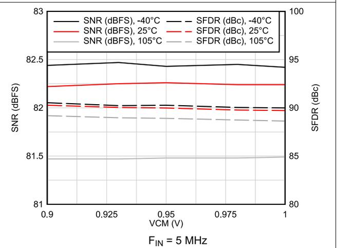
Figure 6-57. AC Performance vs VCM vs Temperature
