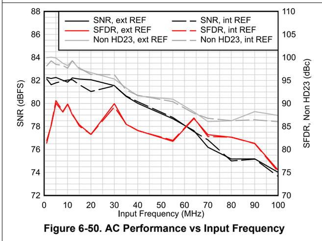
Figure 6-50. AC Performance vs Input Frequency
