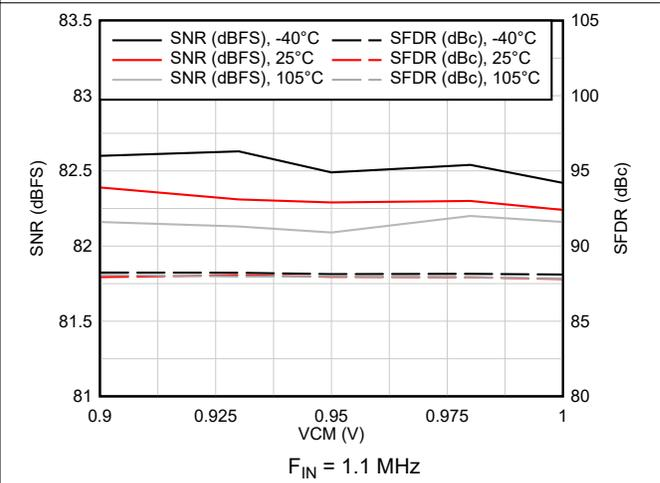
Figure 6-33. AC Performance vs VCM vs Temperature
