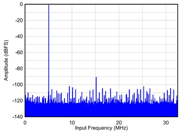
**Figure 6-41. Single Tone FFT at  $F_{IN} = 5\text{ MHz}$**
