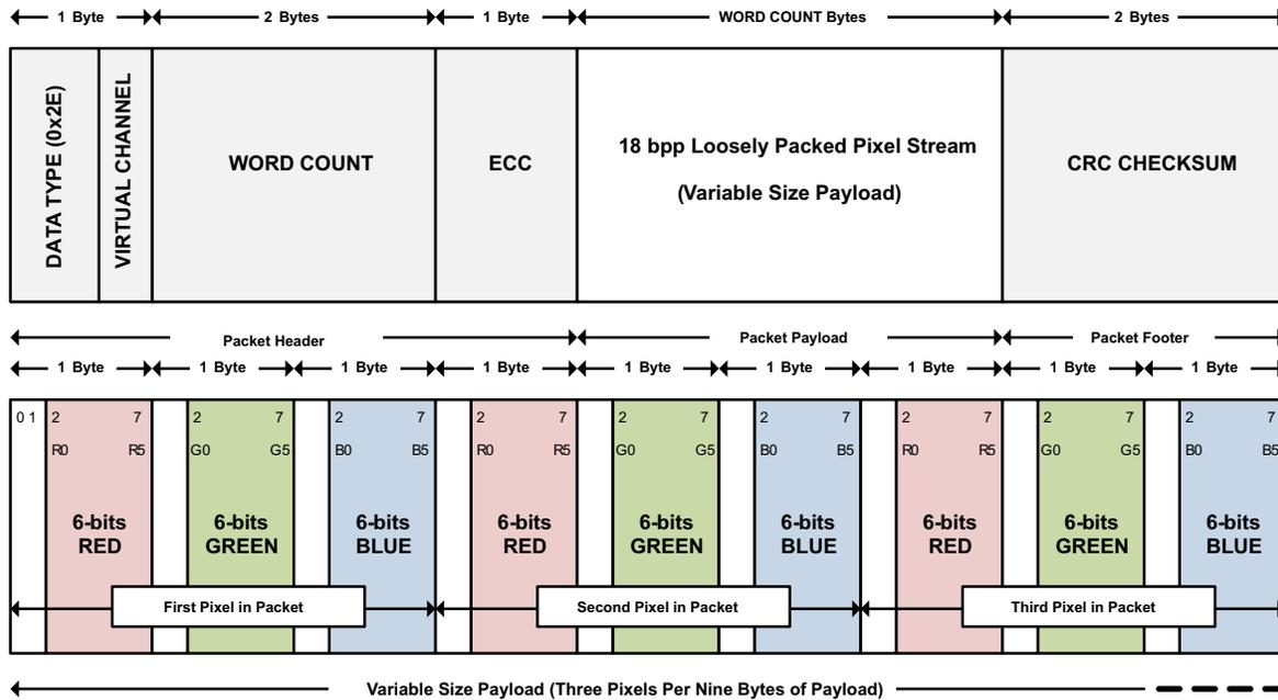
Figure 14. 18-bpp (Loosely Packed) DSI Packet Structure
