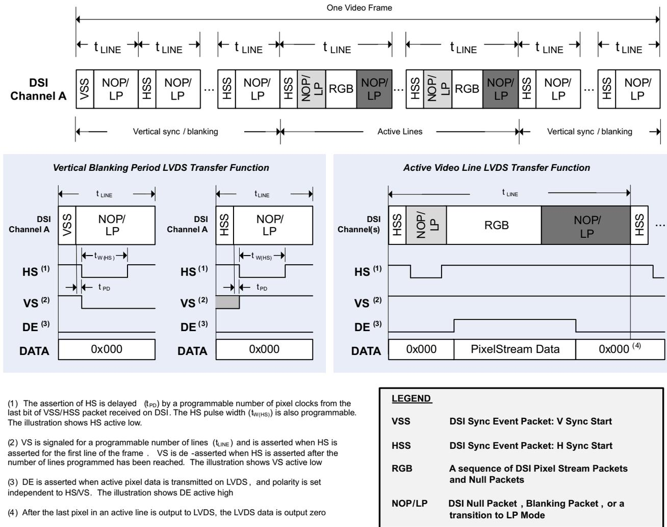
Figure 17. DSI Channel Transmission and Transfer Function
