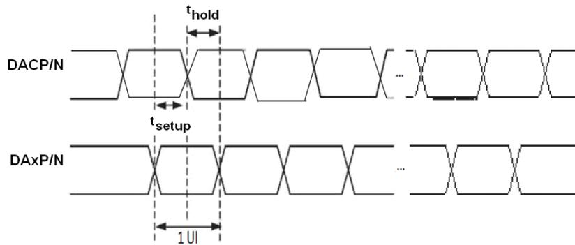
Figure 1. DSI HS Mode Receiver Timing Definitions
