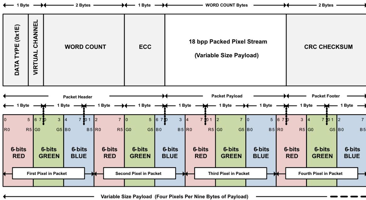
Figure 15. 18-bpp (Tightly Packed) DSI Packet Structure
