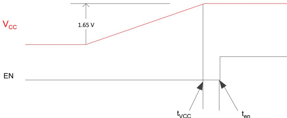
Figure 6. Cold-Start V<sub>CC</sub> Ramp Up to EN
