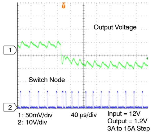
Figure 14. Load Transient
