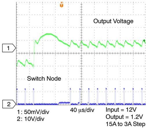
Figure 15. Load Transient
