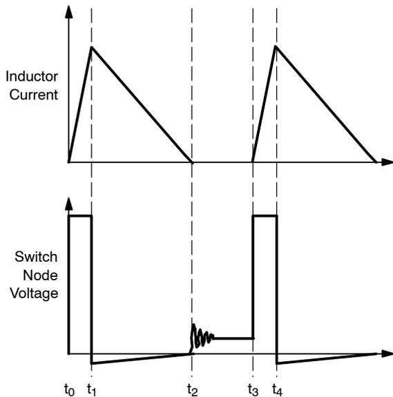
Figure 30. Inductor Current and Switch Node in DCM
