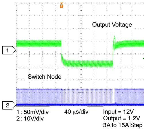
Figure 13. Load Transient
