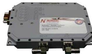
**The NuPower Xtender™ C10RX03 is a small, highly efficient, solid state bidirectional amplifier (BDA) that provides at least 8 watts of RF power across the 4.4 to 5.1 GHz frequency range to boost performance of data links and transmitters.**
