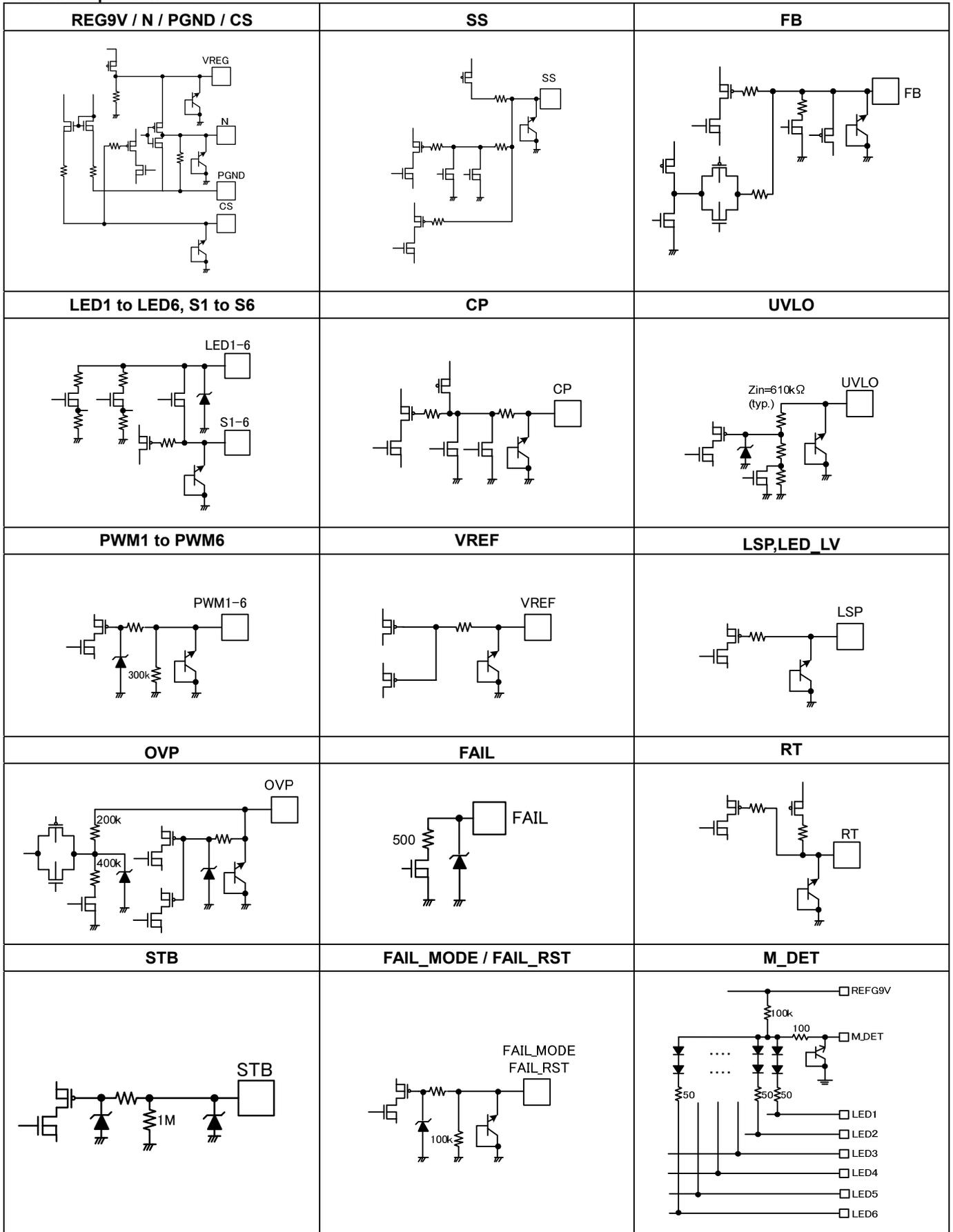
Figure 5. I/O equivalence circuit
