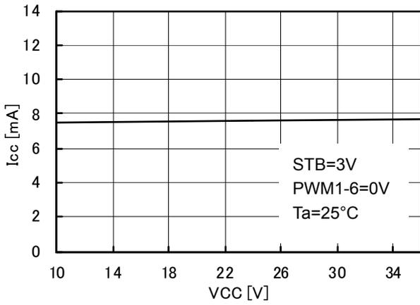
Figure 6. Circuit current
