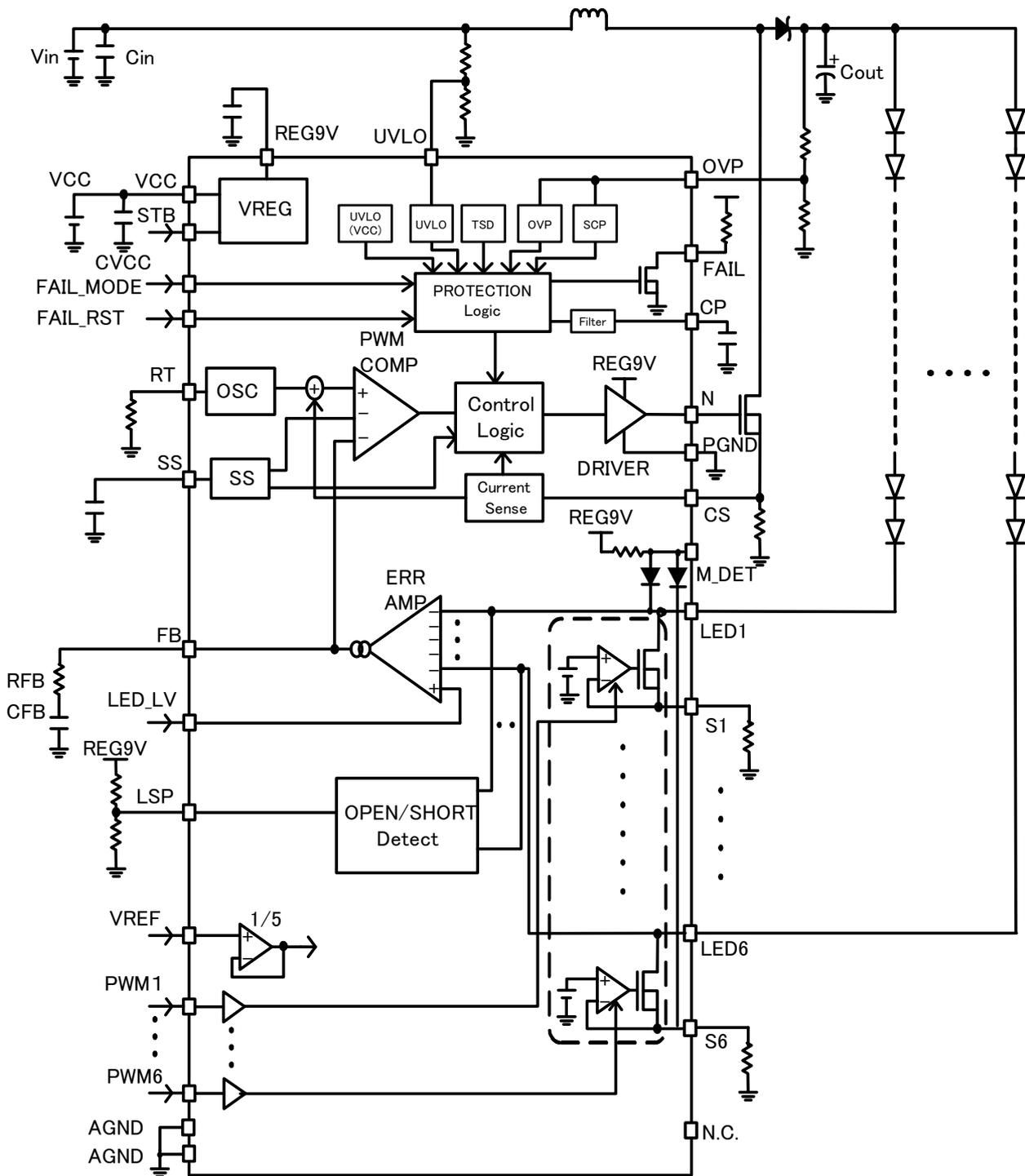
Figure 11. Block Diagram
