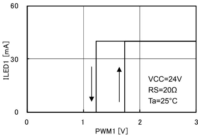
Figure 10. PWM terminal threshold voltage
