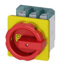
SENTRON, Switch disconnector 3LD, emergency switching-off switch, 3-pole, Iu: 125 A, operating power / at AC-23 A 400 V: 45 kW, front-mounted, rotary operating mechanism, Red / yellow, 4-hole mounting of the handle
