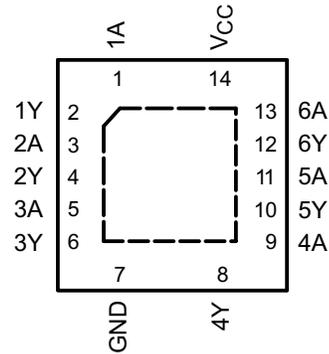
**Figure 5-2. SN74AHCT14 RGY Package, 14-Pin VQFN (Top View)**
