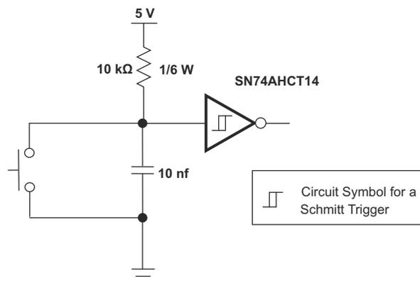
Figure 9-1. Switch De-Bouncer Using Schmitt Trigger Inverter
