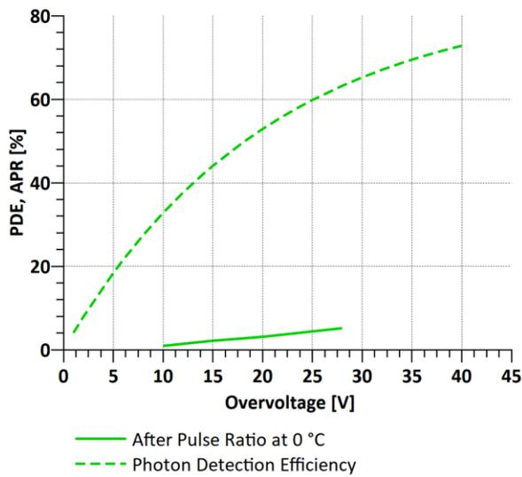
Figure 10: Typical Noise Parameter
