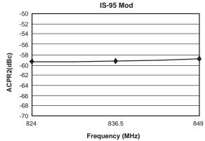
RMPA0967 Cellular 3x3mm<sup>2</sup> PAM Vcc=3.4 V, Vref=2.85V, Vmode=0V, Pout=28 dBm,
