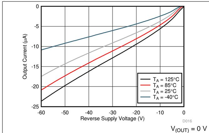
Figure 13. Output Current vs Reverse Supply Voltage,  $-V_{(IN)}$
