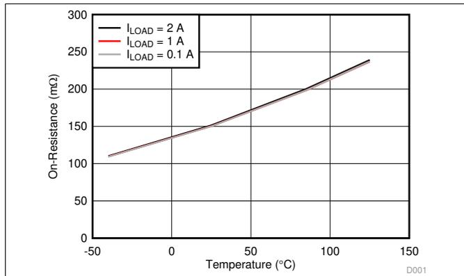
Figure 1. On-Resistance vs Temperature Across Load Current
