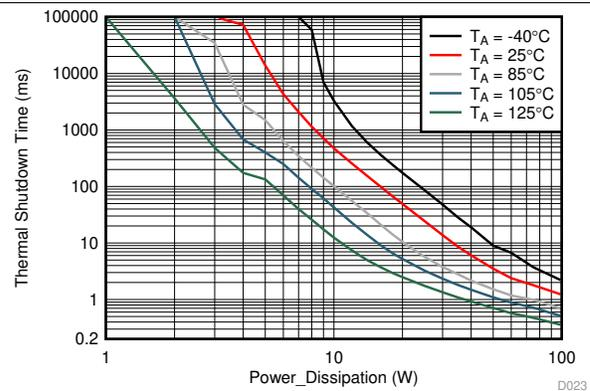
Taken on 2-Layer board, 2 oz.(0.08-mm thick) with HTSSOP device with RTN plane area: 1 cm<sup>2</sup> (Top) and 4.6 cm<sup>2</sup> (Bottom)
