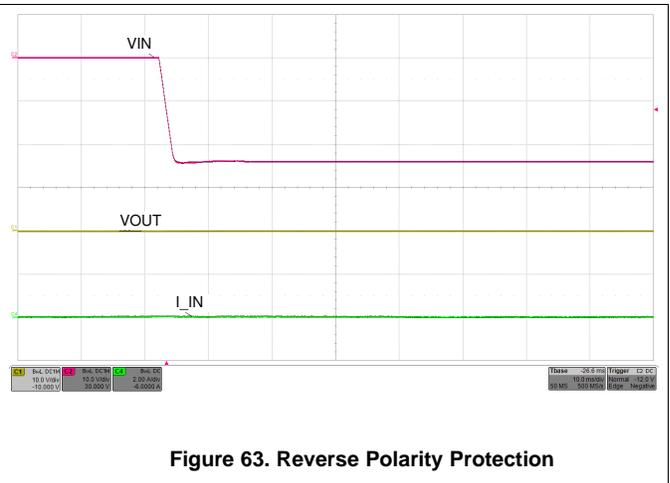
Figure 63. Reverse Polarity Protection
