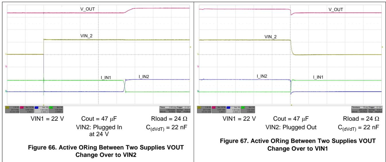
Figure 66. Active ORing Between Two Supplies VOUT Change Over to VIN2
