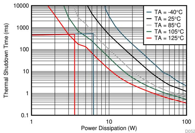
Figure 55. Thermal Shutdown Time vs Power Dissipation
