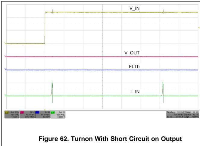
Figure 62. Turnon With Short Circuit on Output
