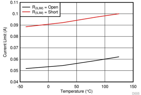
Figure 22. Current Limit for  $R_{(ILIM)} = \text{Open}$  and Short vs Temperature
