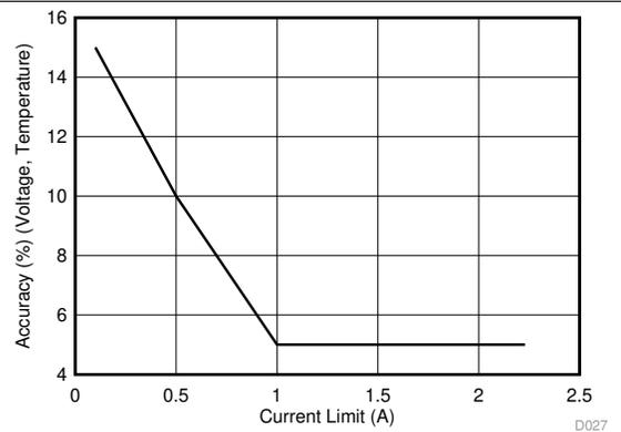
Figure 24. Current Limit Accuracy vs Current Limit,  $I_{(OL)}$
