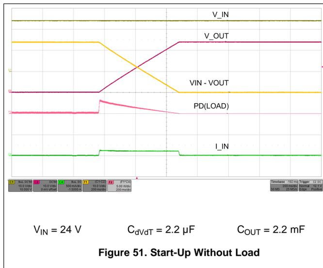
Figure 51. Start-Up Without Load
