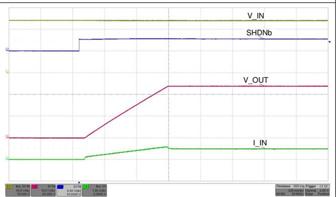
Figure 59. Start-Up With Shutdown Pin—48-Ω Load
