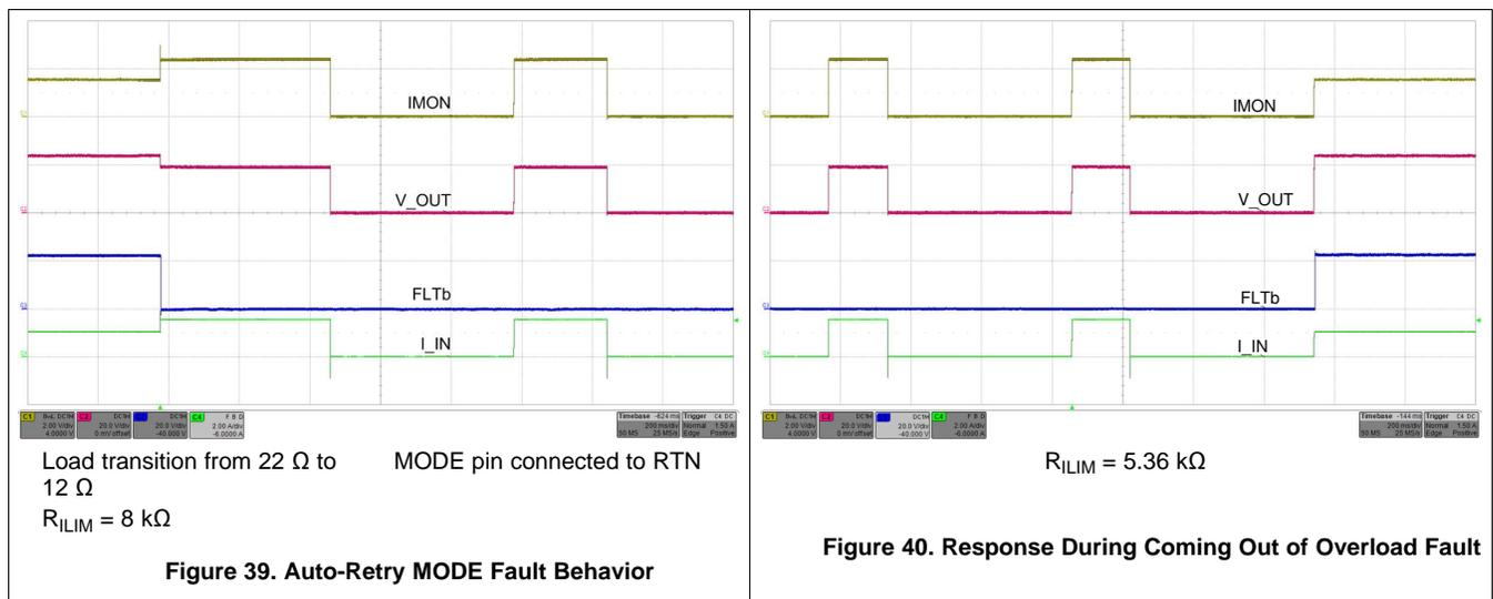
9.3.5.1.2 Electronic Circuit Breaker with Overload Timeout, MODE = OPEN
