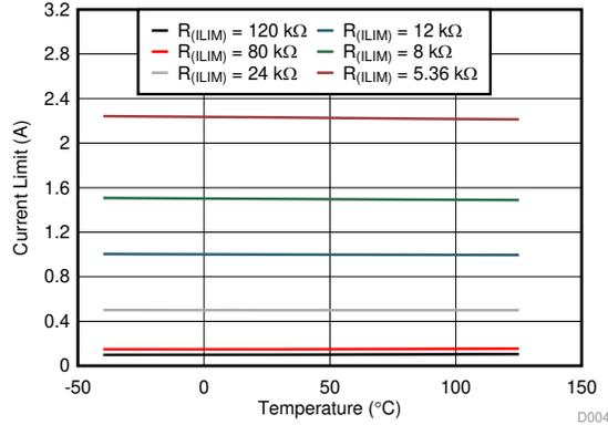
Figure 21. Over Load Current Limit vs Temperature
