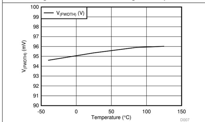
Figure 5.  $V_{(FWDTH)}$  vs Temperature
