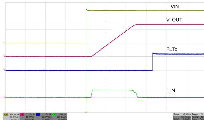
$$C_{dVdT} = 22 \text{ nF} \quad C_{OUT} = 47 \mu\text{F} \quad R_{LIM} = 5.36 \text{ k}\Omega$$
