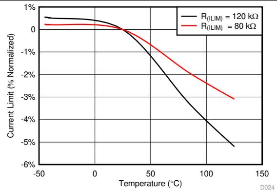
Figure 20. Current Limit (% Normalized) vs Temperature
