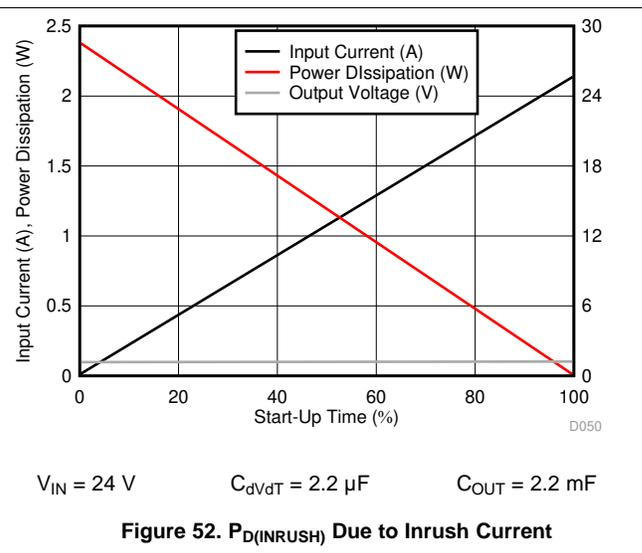
Figure 52.  $P_{D(INRUSH)}$  Due to Inrush Current
