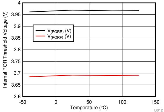
Figure 9. Internal POR Threshold Voltage vs Temperature
