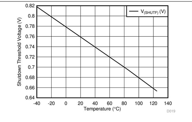
Figure 16. Shutdown Threshold Voltage Shutdown vs Temperature
