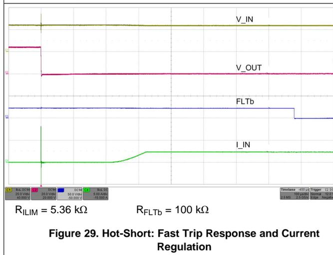
Figure 29. Hot-Short: Fast Trip Response and Current Regulation
