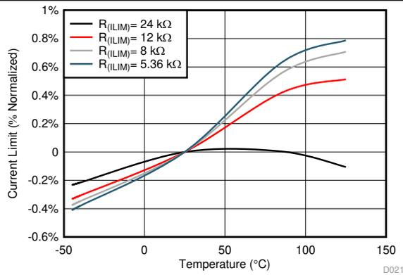
Figure 19. Current Limit (% Normalized) vs Temperature
