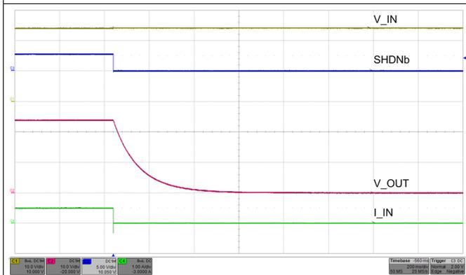
Figure 60. Power Down With Shutdown Pin—48-Ω Load
