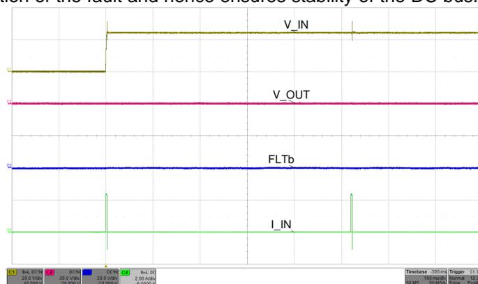
MODE pin connected to RTN
