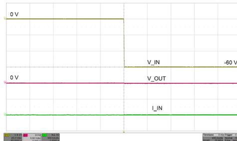
Figure 36. Reverse Input Supply Protection at -60 V
