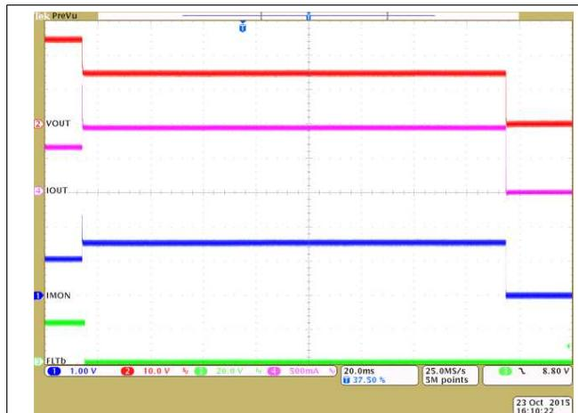
Figure 46. Look Ahead Overload Current Fault Indication
