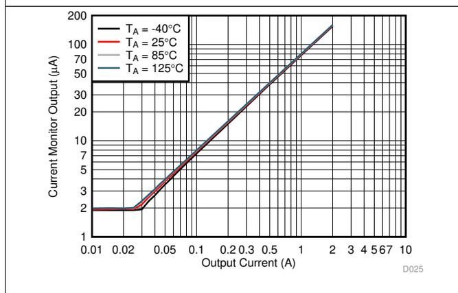
Figure 17. Current Monitor Output vs Output Current
