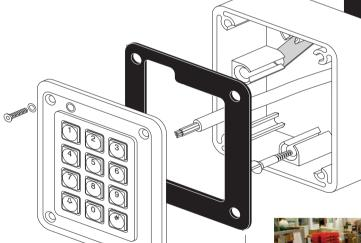
(Fixing hardware, sealing gaskets and comprehensive installation / operating instructions are included)
