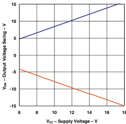
Figure 5. Output Voltage Swing vs Supply Voltage
