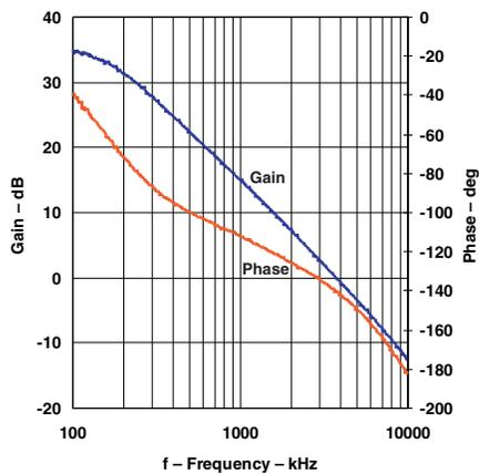
Figure 3. Gain and Phase vs Frequency
