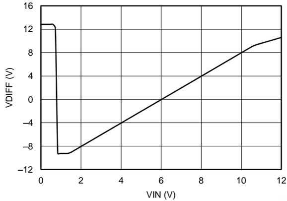
Figure 15. Differential Output Voltage Node vs Input Voltage
