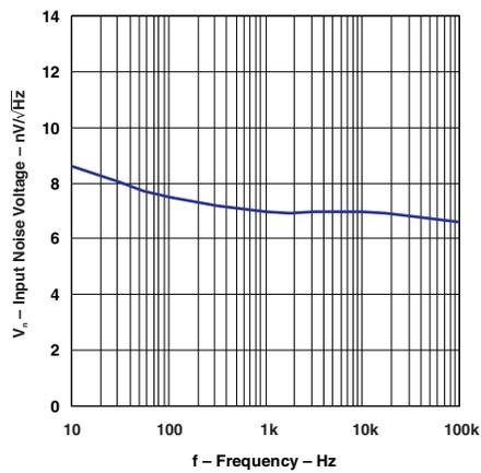
**Figure 13. Input Noise Voltage vs Frequency**
