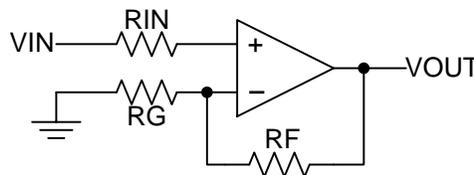
Figure 18. Operational Amplifier Schematic for Noninverting Configuration
