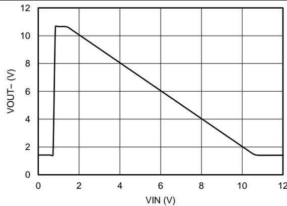
Figure 17. Positive Output Voltage Node vs Input Voltage
