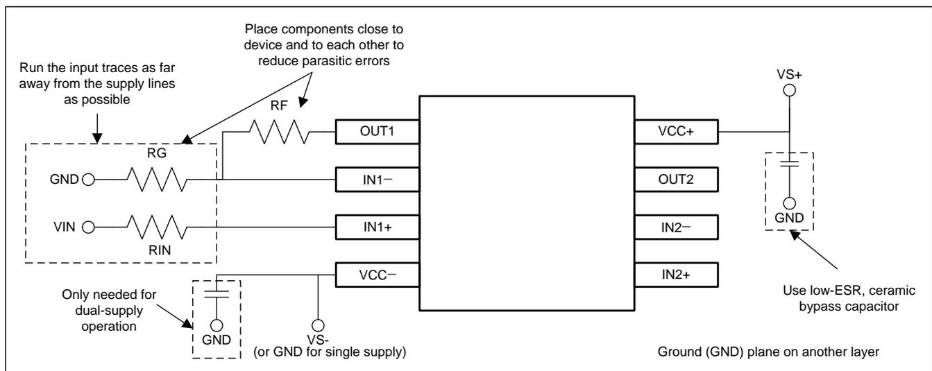
Figure 19. Operational Amplifier Board Layout for Noninverting Configuration
