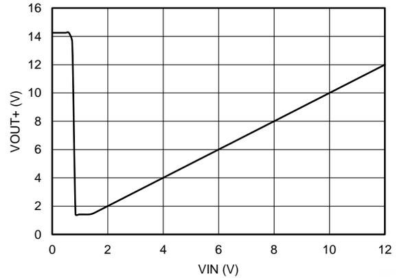
Figure 16. Positive Output Voltage Node vs Input Voltage
