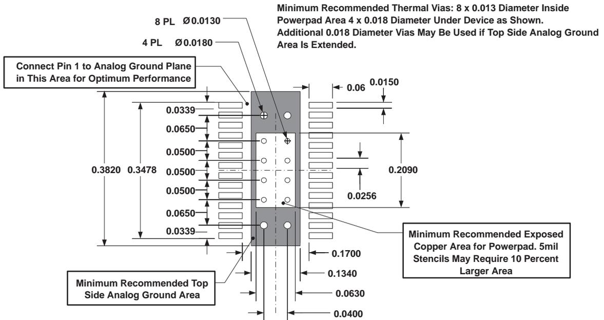
Figure 11. Recommended Land Pattern for 28-Pin PWP PowerPAD
