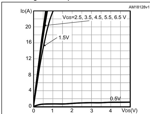
Figure 5. Transfer characteristics
