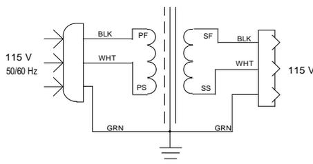
\* Leakage current between primary and secondary is typically measured at less than 10µA.
