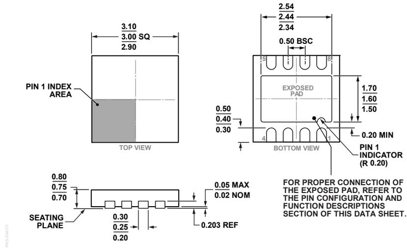
Figure 66. 8-Lead Lead Frame Chip Scale Package [LFCSP\_WD]
