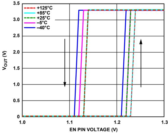
Figure 50. Typical VOUT Response to EN Pin Operation
