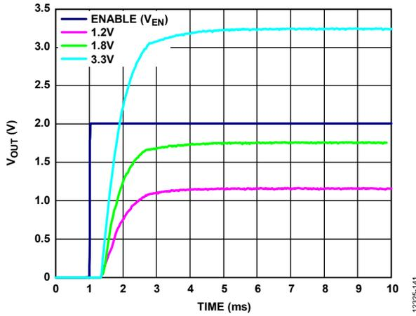
Figure 41.  $V_{OUT}$  Start-Up Time After  $V_{EN}$  Rising, Different Output Voltages,  $V_{IN} = 5V$
