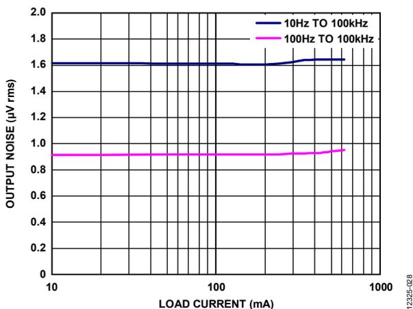
Figure 28. RMS Output Noise vs. Load Current ( $I_{LOAD}$ )
