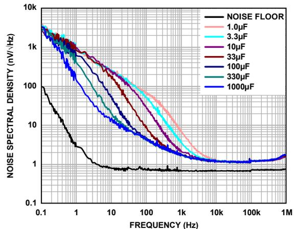
Figure 2. Noise Spectral Density for Different Values of  $C_{\text{BYVP}}$
