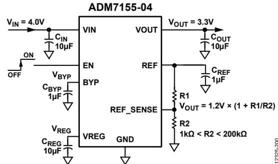
Figure 43. Typical Adjustable Output Voltage Application Schematic
