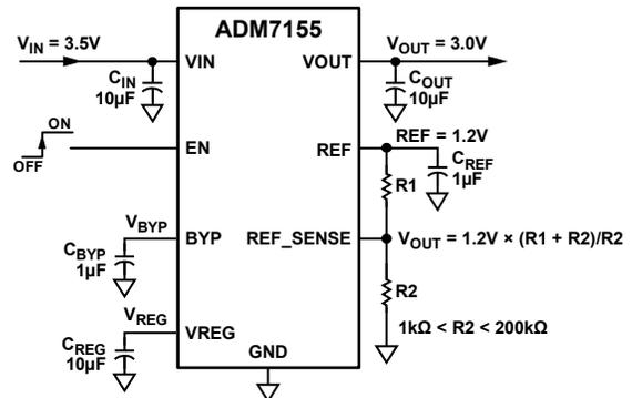
Figure 1. Regulated 3.0V Output from 3.5V Input
