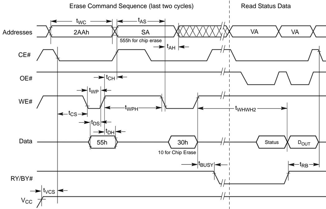
**Figure 22. Back-to-back Read/Write Cycle Timings**
