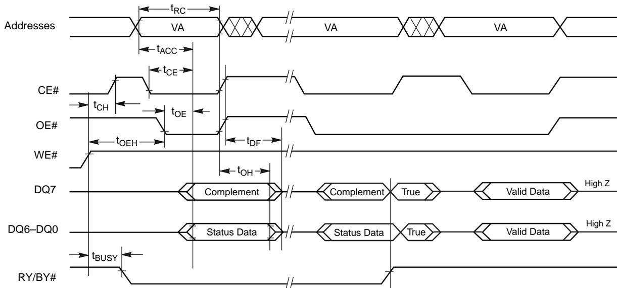
Figure 24. Toggle Bit Timings (During Embedded Algorithms)<sup>[77]</sup>
