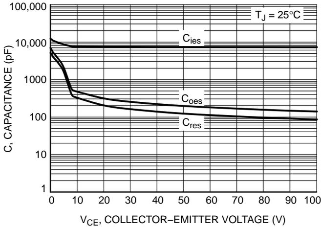
Figure 3. Typical Capacitance
