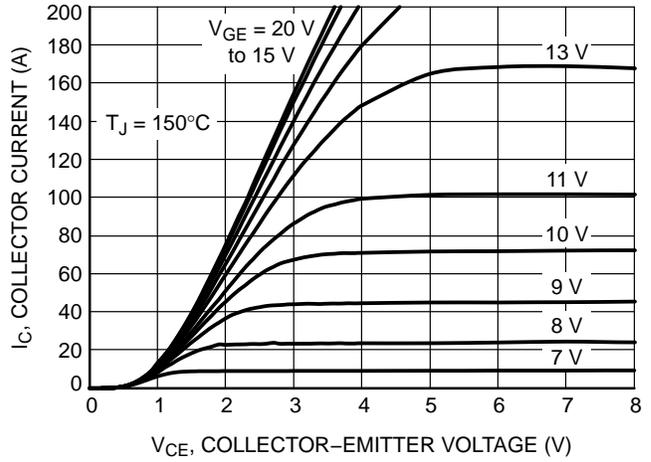
Figure 2. Output Characteristics
