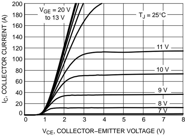
Figure 1. Output Characteristics
