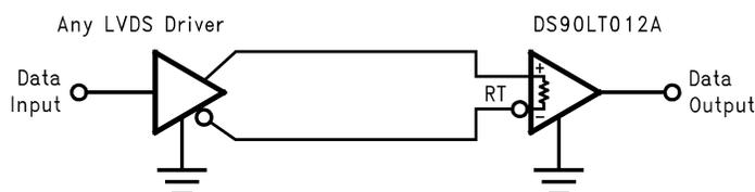
**Figure 5. Balanced System — Point-to-Point Application (DS90LT012AQ)**
