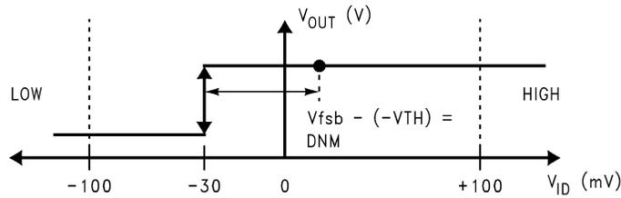
**Figure 6. VTC of the DS90LT012AQ LVDS Receiver**
