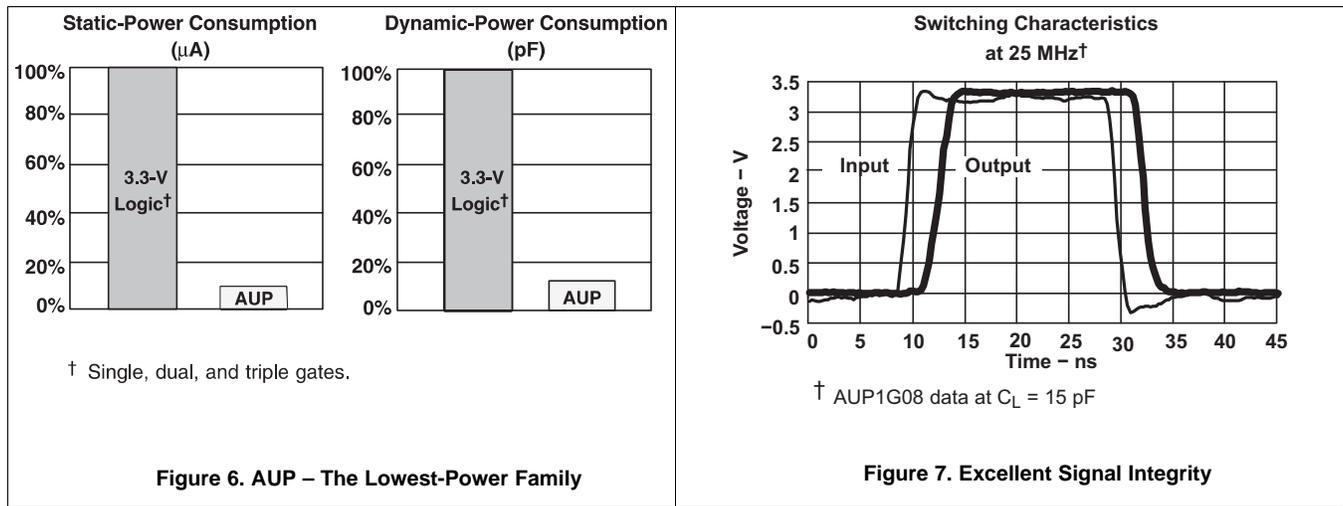
The AUP family of single gate logic makes excellent translators for the new lower voltage microprocessors that typically are powered from 0.8 V to 1.2 V. They can drop the voltage of peripheral drivers and accessories that are still powered by 3.3 V to the new uC power levels.
