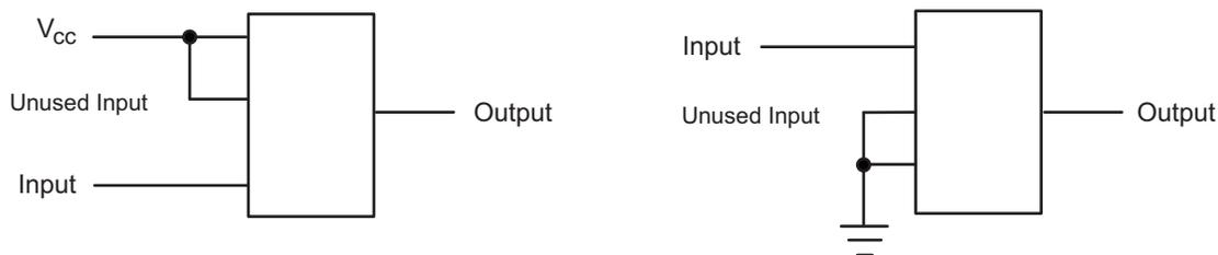
**Figure 8. Layout Diagram**
